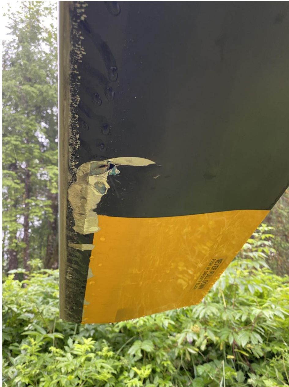
Photo 2 – Additional picture of damaged blade (Photo courtesy of the operator)
