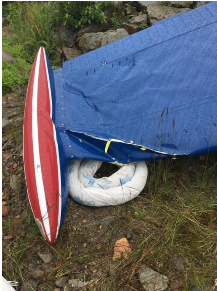
Photo 2 - View of damaged right wing (Photo courtesy of the operator)
