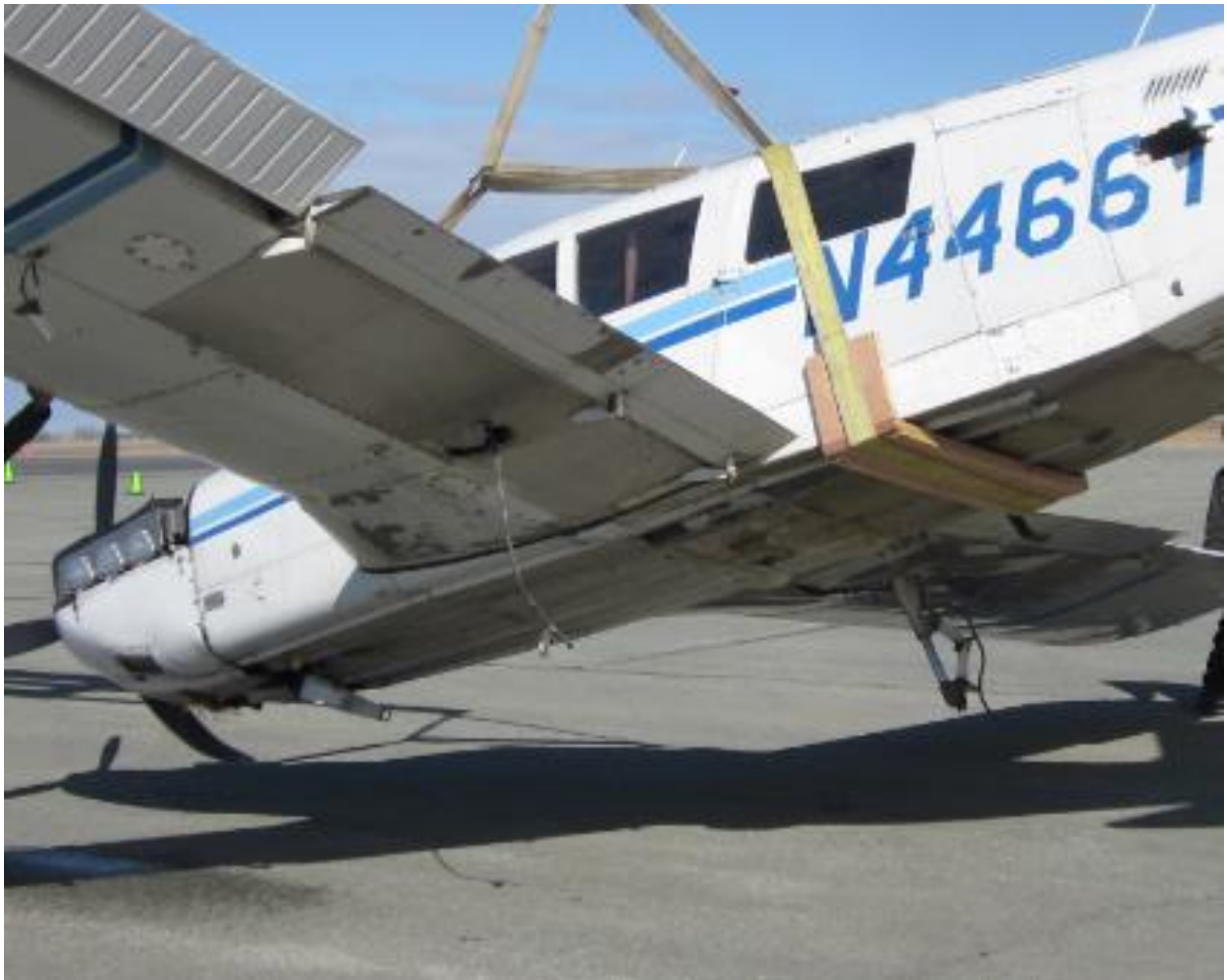
Photo 1 – View of damaged lower right wing (Photo courtesy of the FAA)
