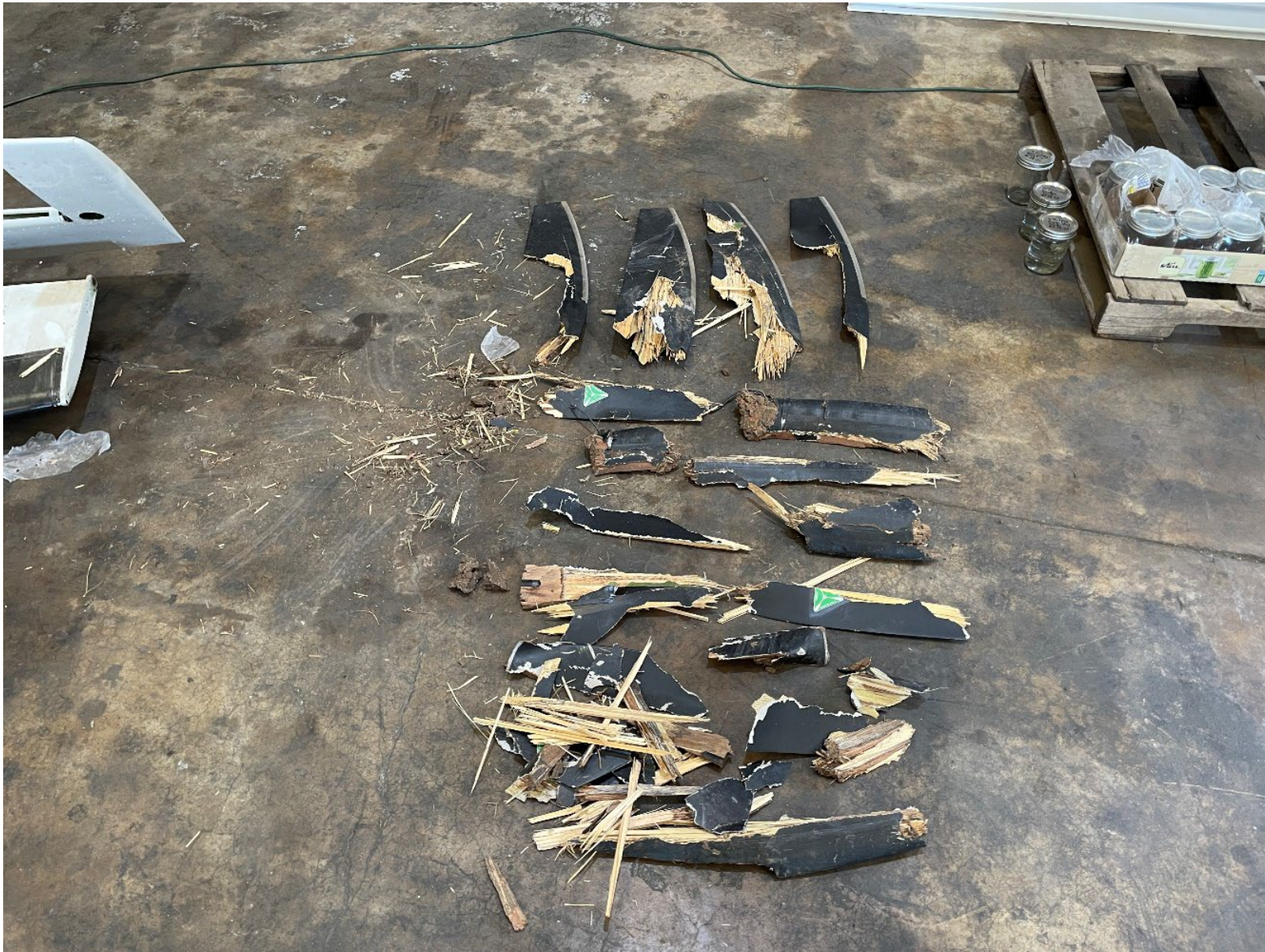
Photograph 12 - View of the propeller blades during the layout.
