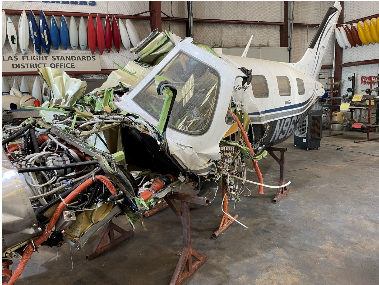
Photograph 8 - View of the airframe during layout.
