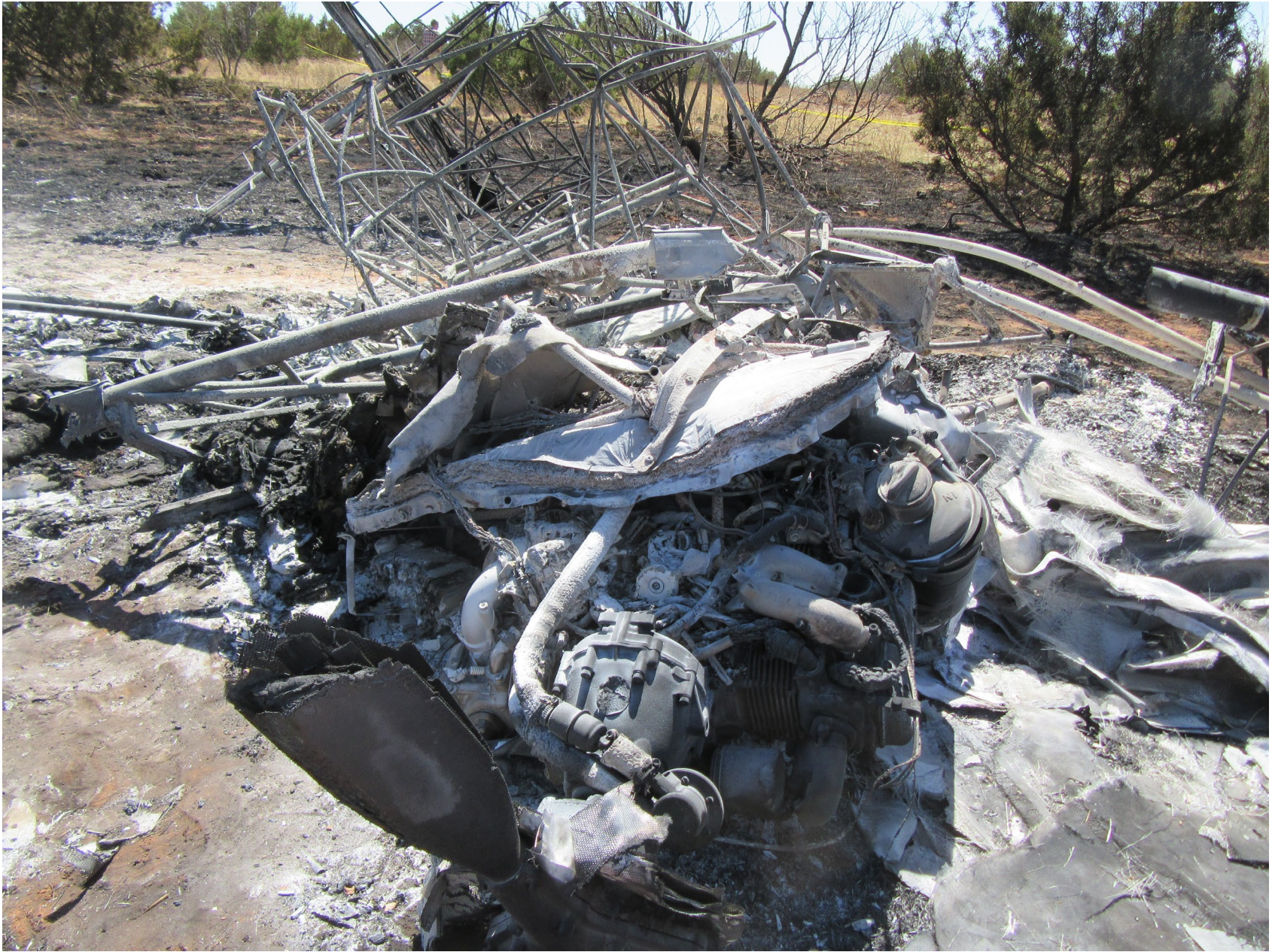
Photo 7 – View of the propeller, the engine, and the cockpit (courtesy of the Federal Aviation Administration).
