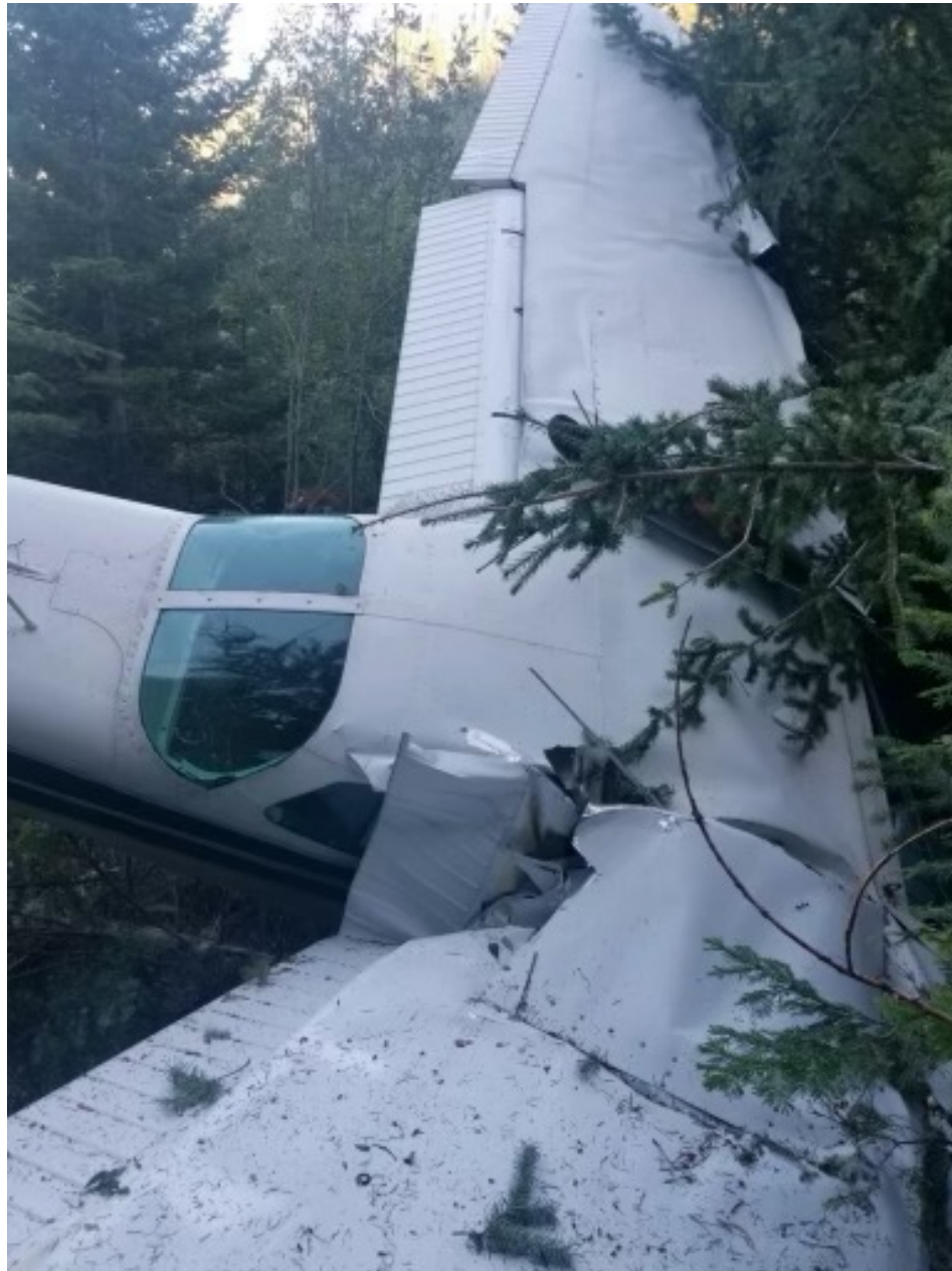
Photo 2 - View of left and right wing damage (photo courtesy of local law enforcement).
