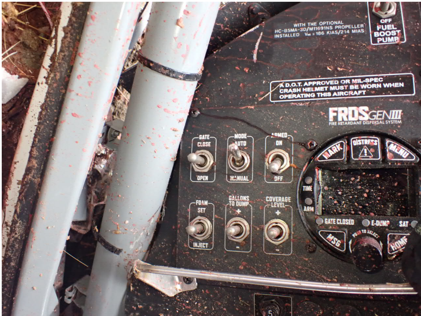
Photo 2 – View of Trotter Controls Gen III Firegate in the off position (photo courtesy of Air Tractor).
