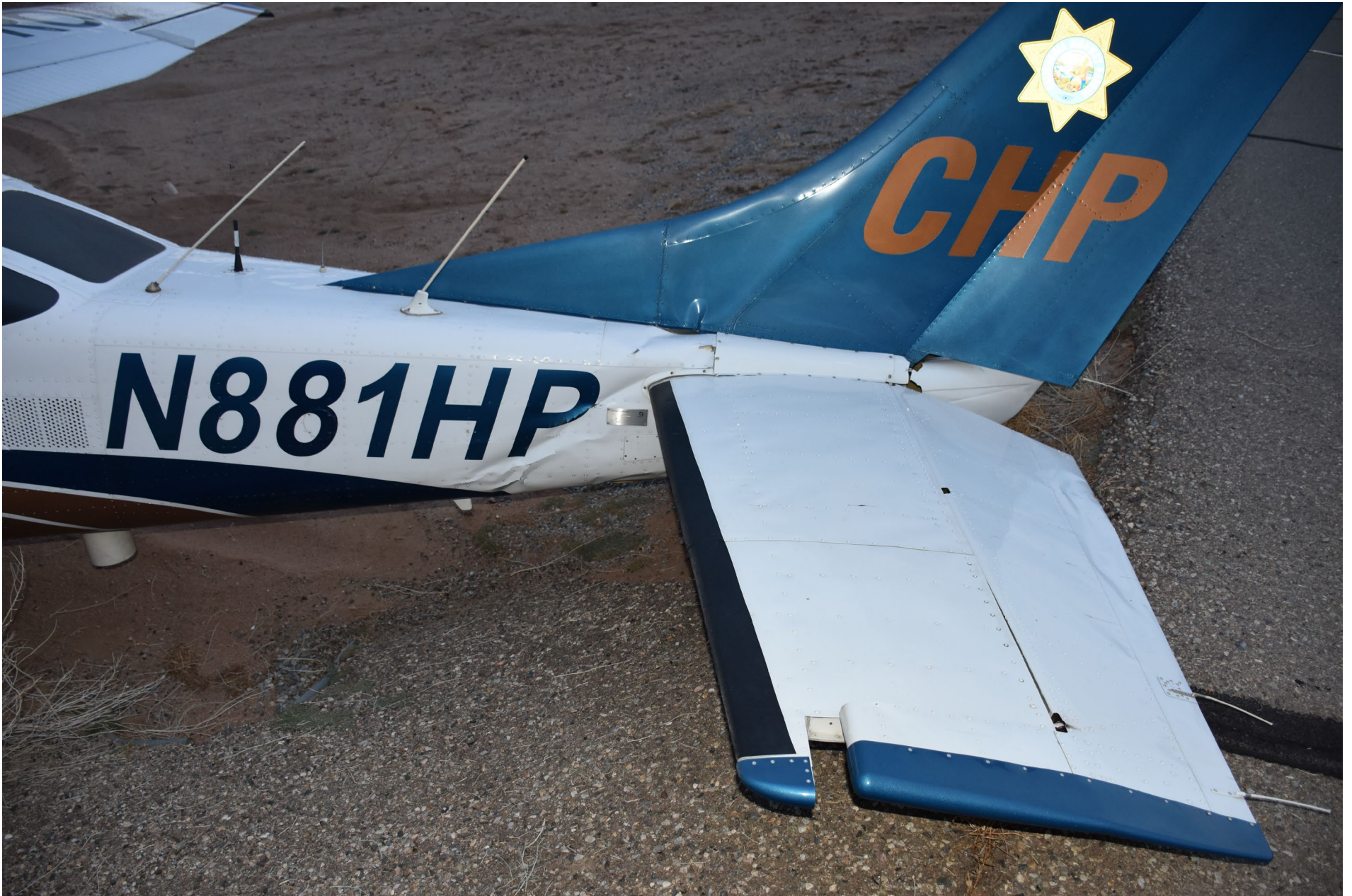
Photo – View of damage to aft section of the fuselage (courtesy of the operator)
