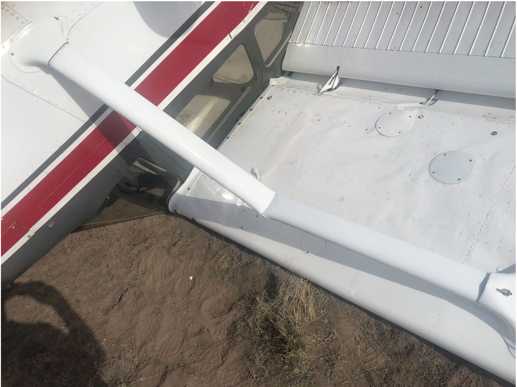
Photo 2 – View of damaged right-wing lift strut (photo courtesy of the pilot)
