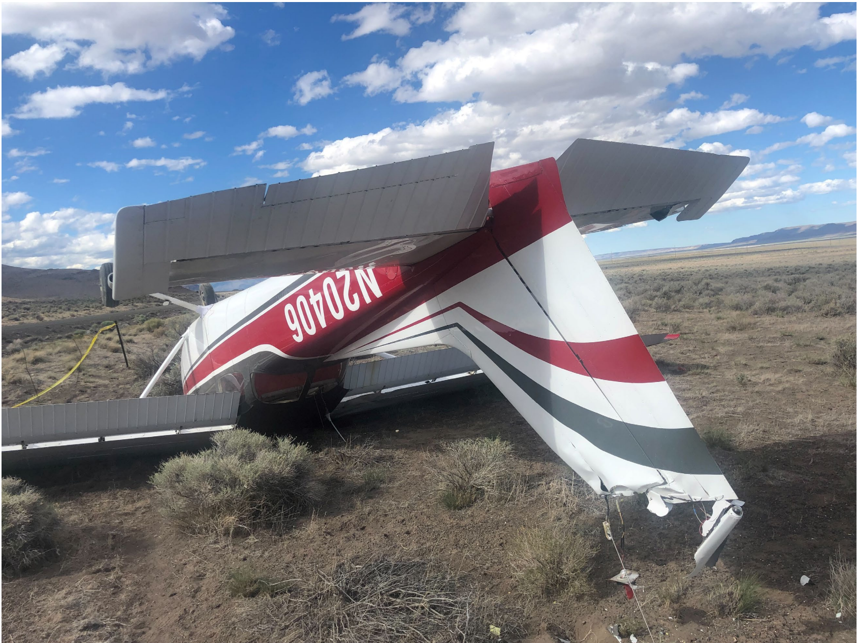
Photo 3 – View of damaged empennage (photo courtesy of the pilot)
