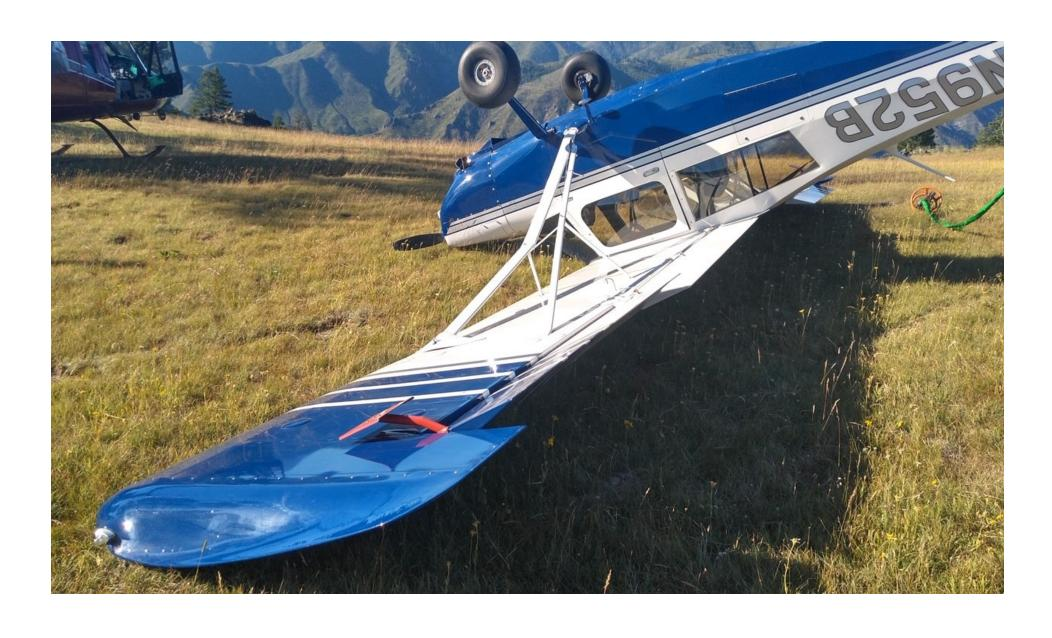
Photo 1 – View of nosed over airplane with damaged right wing lift strut (courtesy of the FAA)
