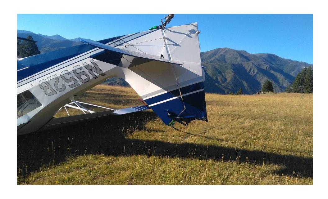
Photo 2 - View of nosed over airplane with damaged rudder (courtesy of the FAA)
