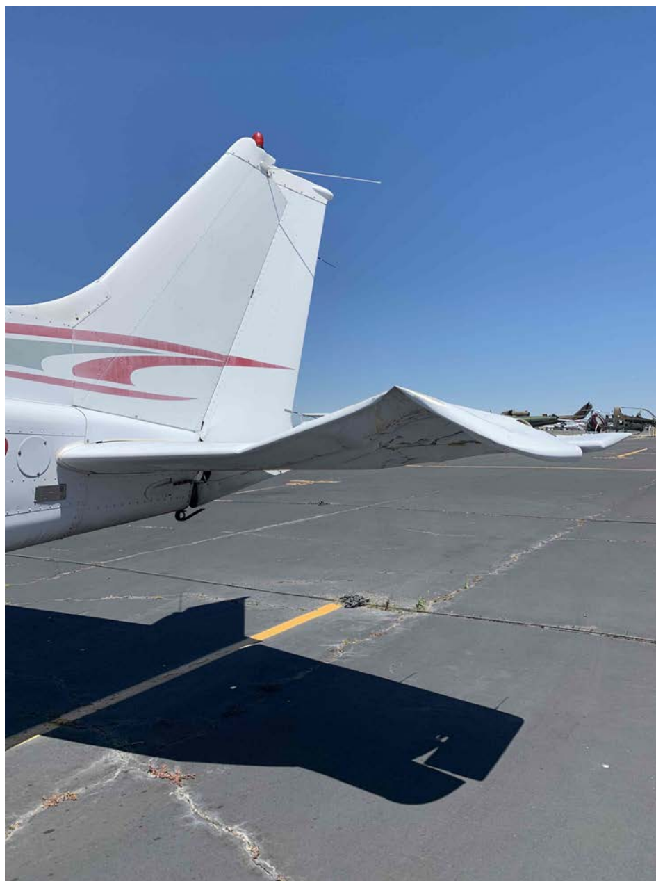
Photo 1 – View of damaged left horizontal stabilizer (courtesy of the FAA)
