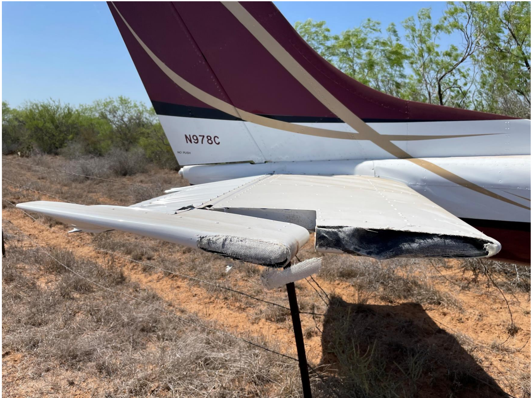
Photo 2 – Right Horizontal Stabilizer / Elevator (Pilot Photo)
