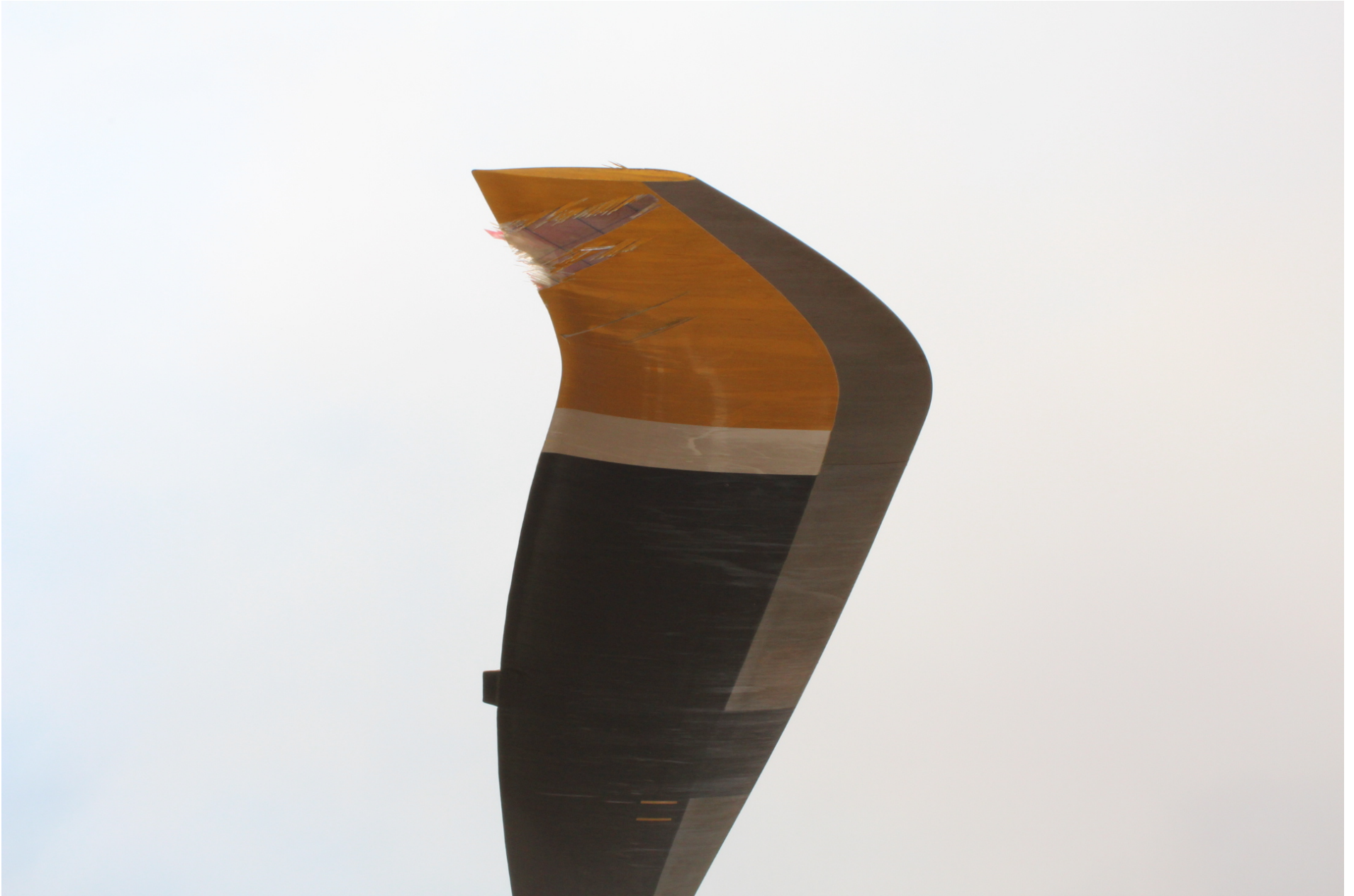
Photo 8 – View of impact damage to the “red” main rotor blade (courtesy of the LAFD).
