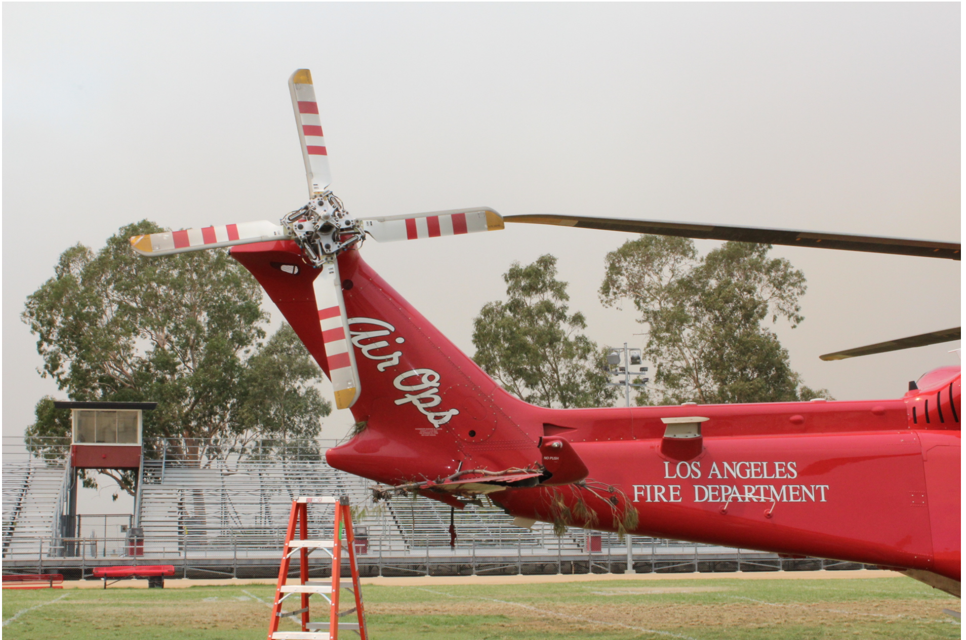
Photo 4 – View of the substantial damage to the empennage with embedded pine tree branches (courtesy of the LAFD).
