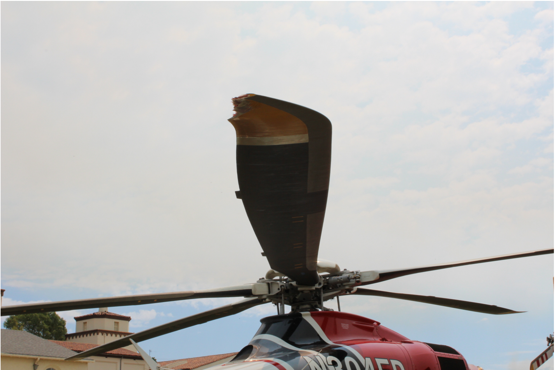
Photo 7 – View of impact damage to the “blue” main rotor blade (courtesy of the LAFD).
