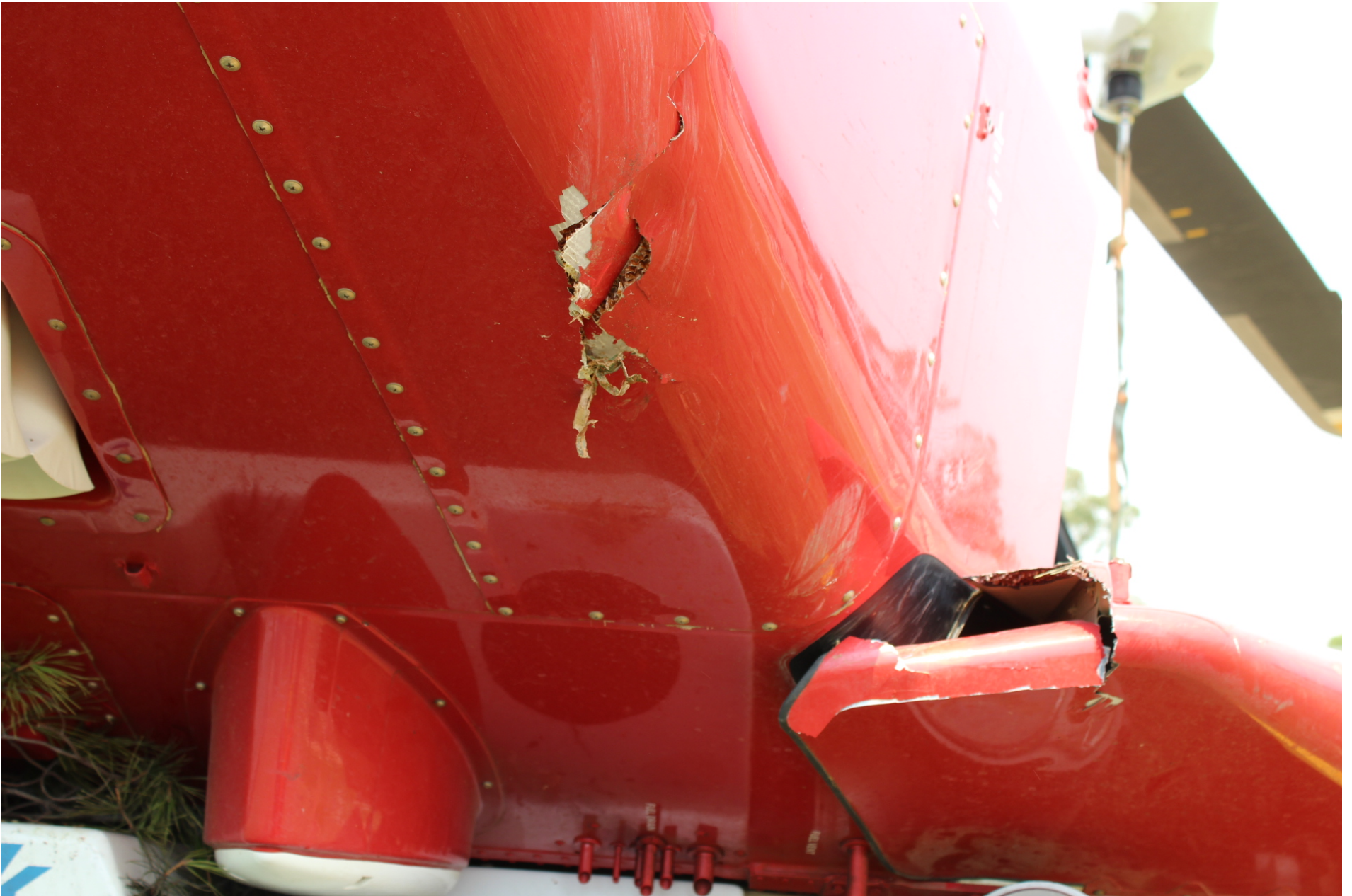
Photo 6 – View of the substantial damage to the tailboom (courtesy of the LAFD).
