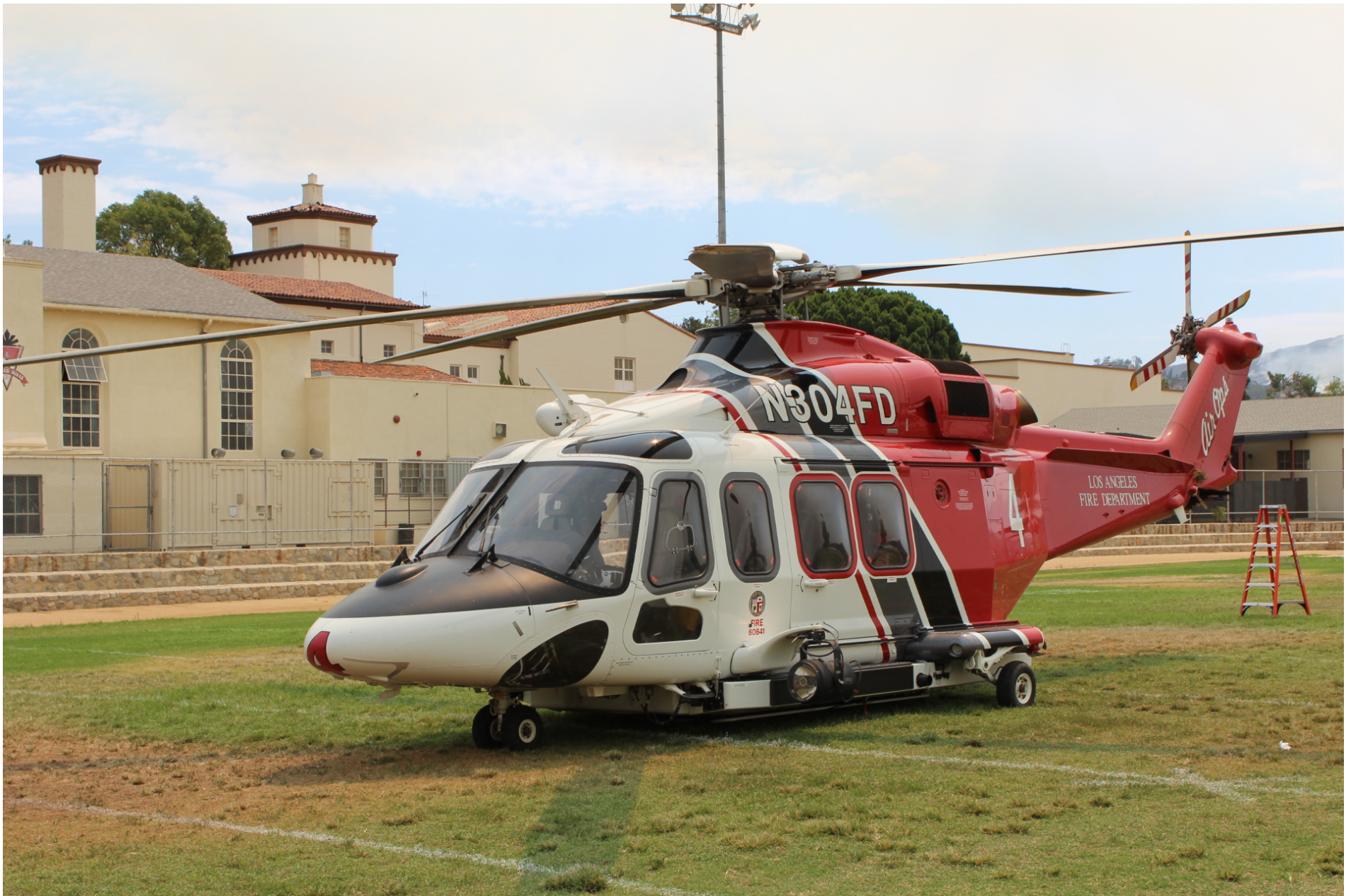
Photo 3 – Postaccident view of the helicopter equipped with the belly-mounted Simplex Aerospace Model 326 GII Fire Attack System (courtesy of the LAFD).
