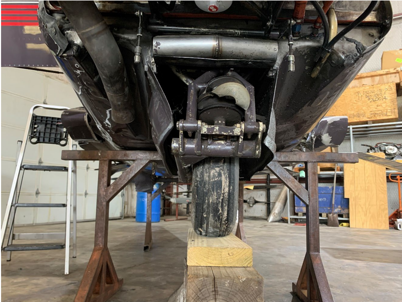
Photograph 18 - View of the underside of the fuselage at the salvage facility, coated with engine oil
