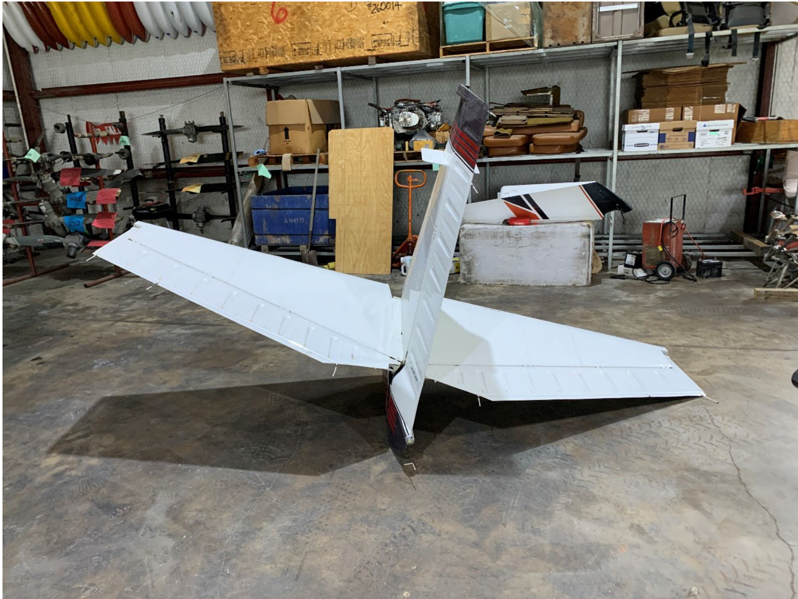
Photograph 14 - View of the empennage at the salvage facility
