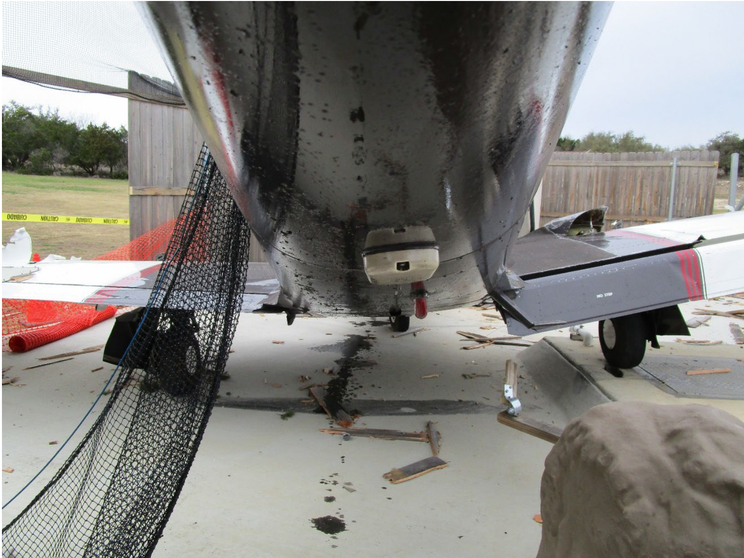
Photograph 8 - View of the underside of the fuselage at the accident site, coated with engine oil (Courtesy of the Federal Aviation Administration)
