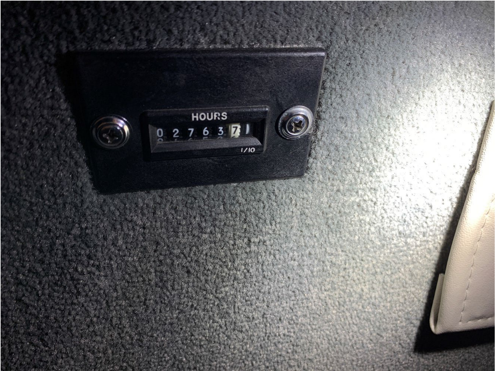
Photograph 20 - View of the Hobbs meter at the salvage facility
