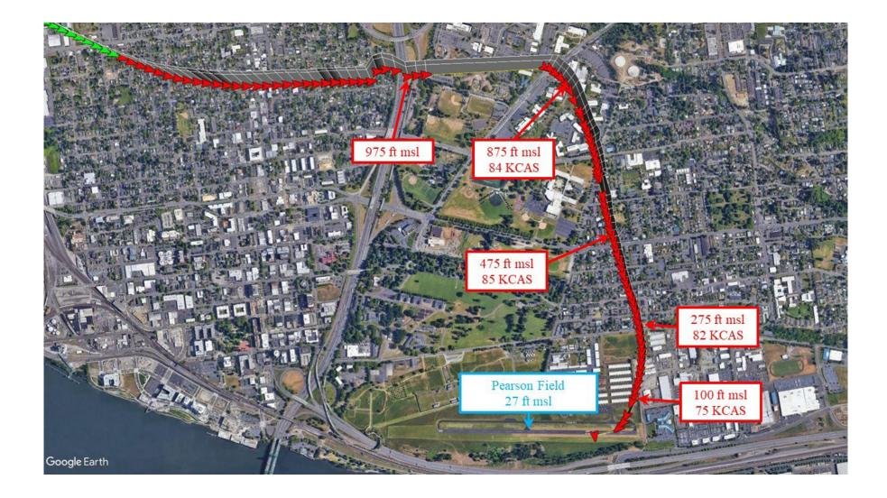
Photo 1 – Figure of altitudes and airspeeds from airplane flight path
