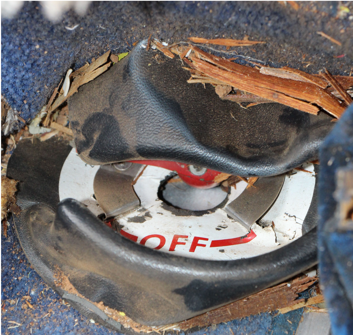
Photo 3 – Fuel selector at accident site
