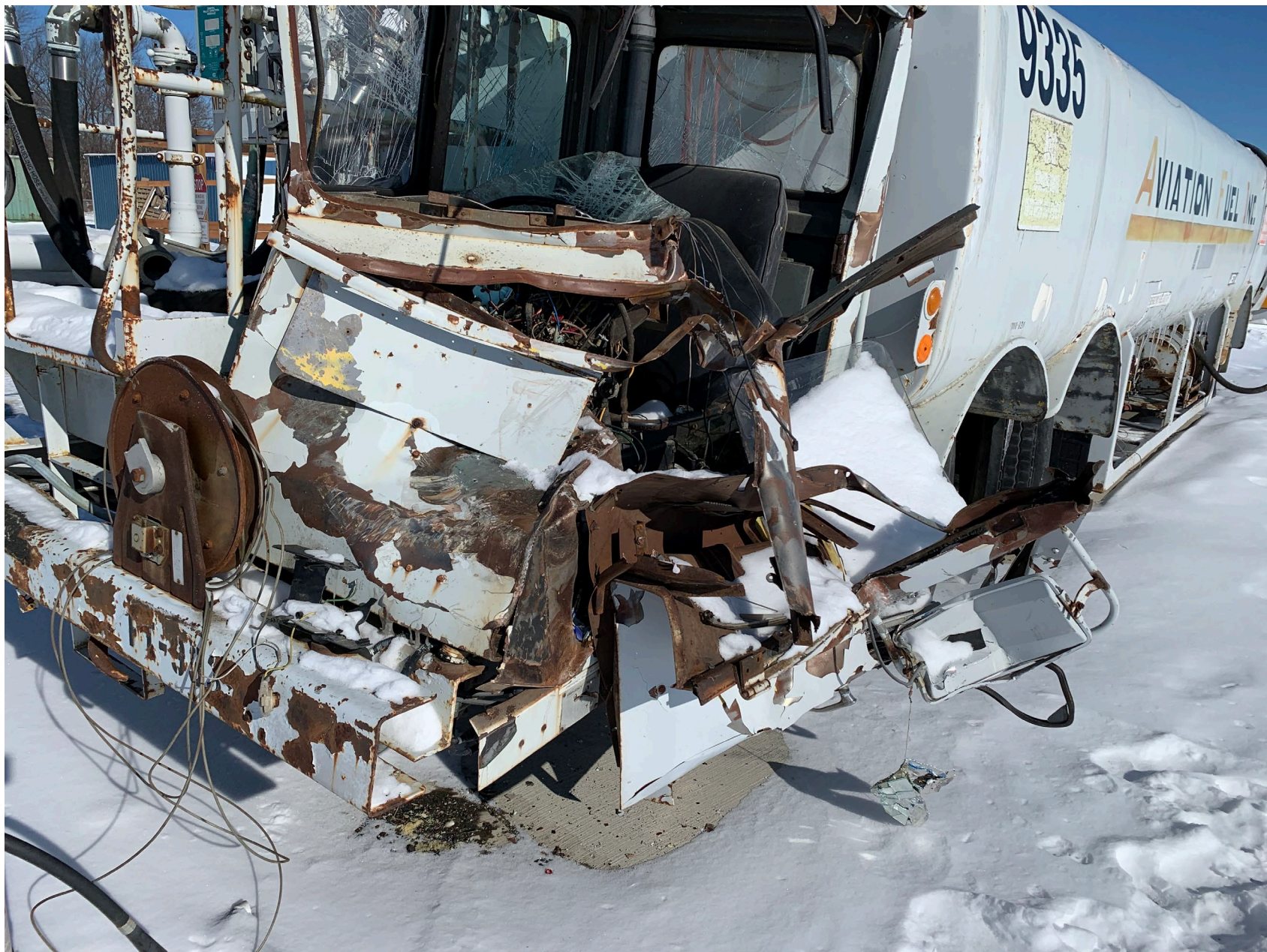
Photo 9 – View of the damage that was sustained to the fuel truck.
