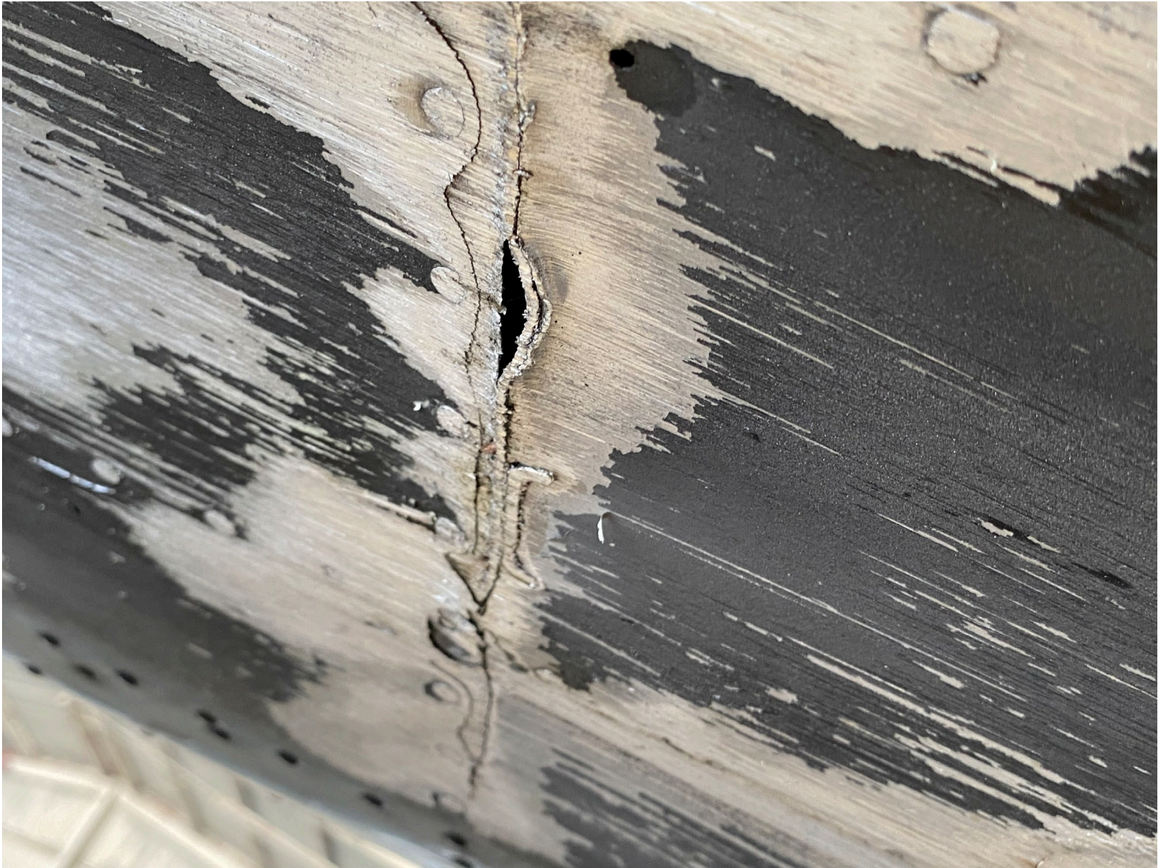
Photo 4 – Closeup view of the substantial damage sustained to the underside of the fuselage (courtesy of the Federal Aviation Administration).
