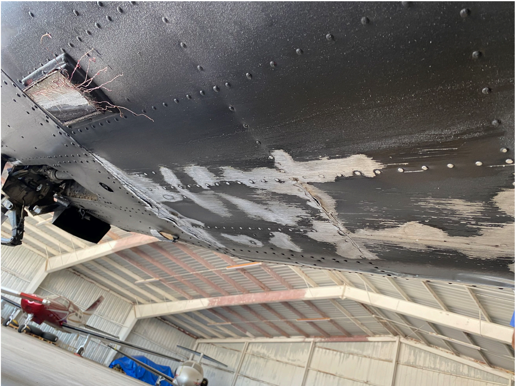
Photo 3 – View of the substantial damage sustained to the underside of the fuselage (courtesy of the Federal Aviation Administration).
