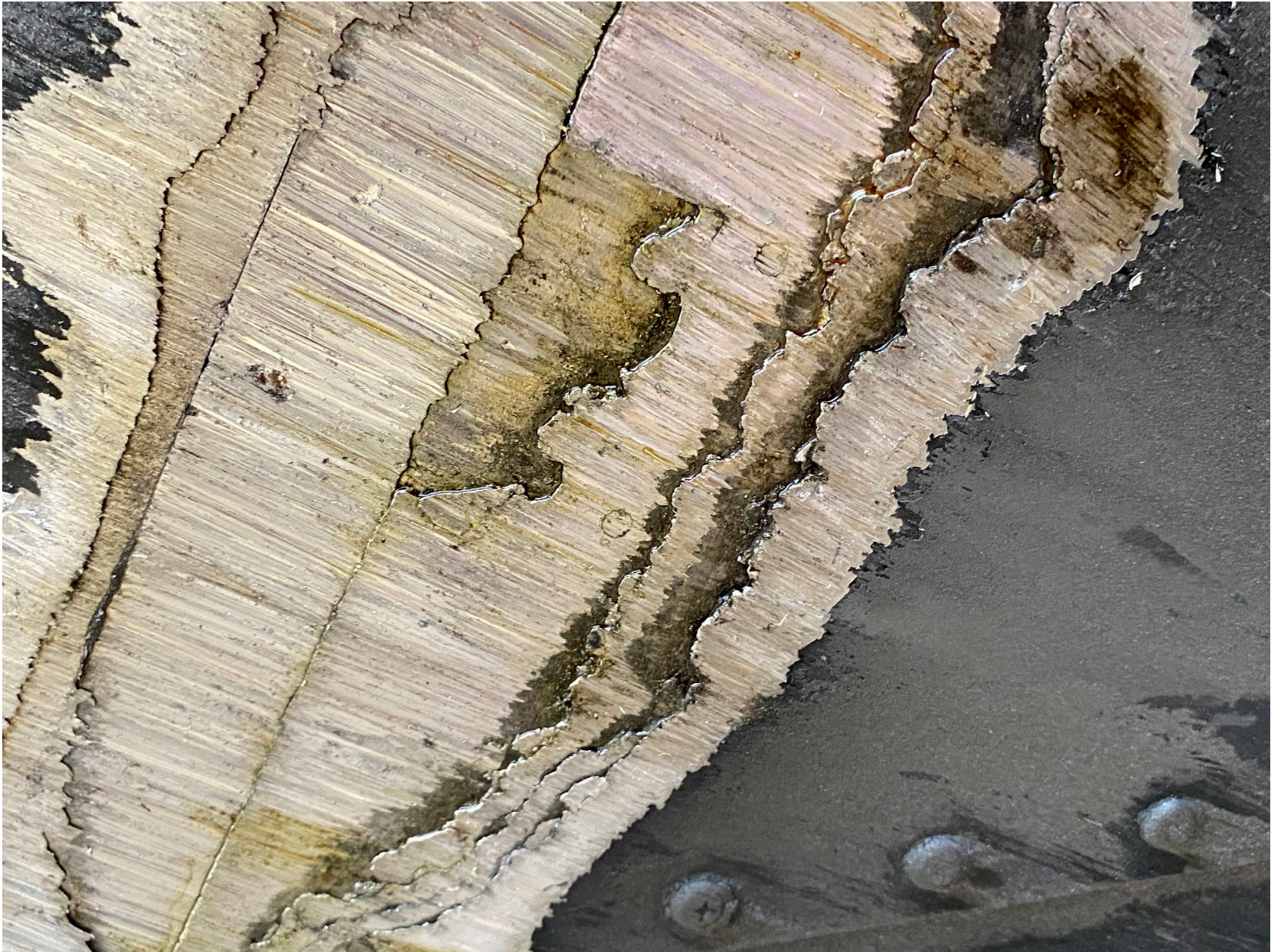
Photo 2 – Closeup view of the substantial damage sustained to the underside of the fuselage (courtesy of the Federal Aviation Administration).
