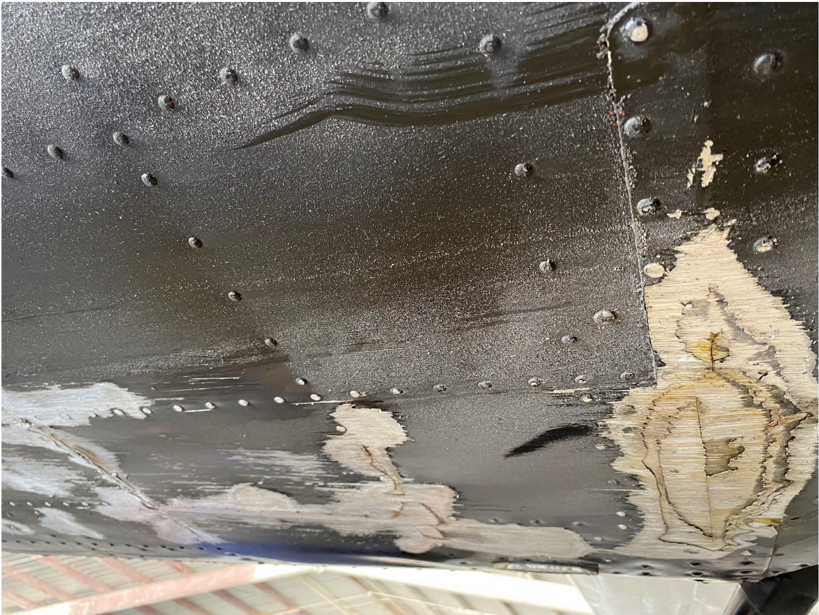
Photo 1 – View of the substantial damage sustained to the underside of the fuselage (courtesy of the Federal Aviation Administration).
