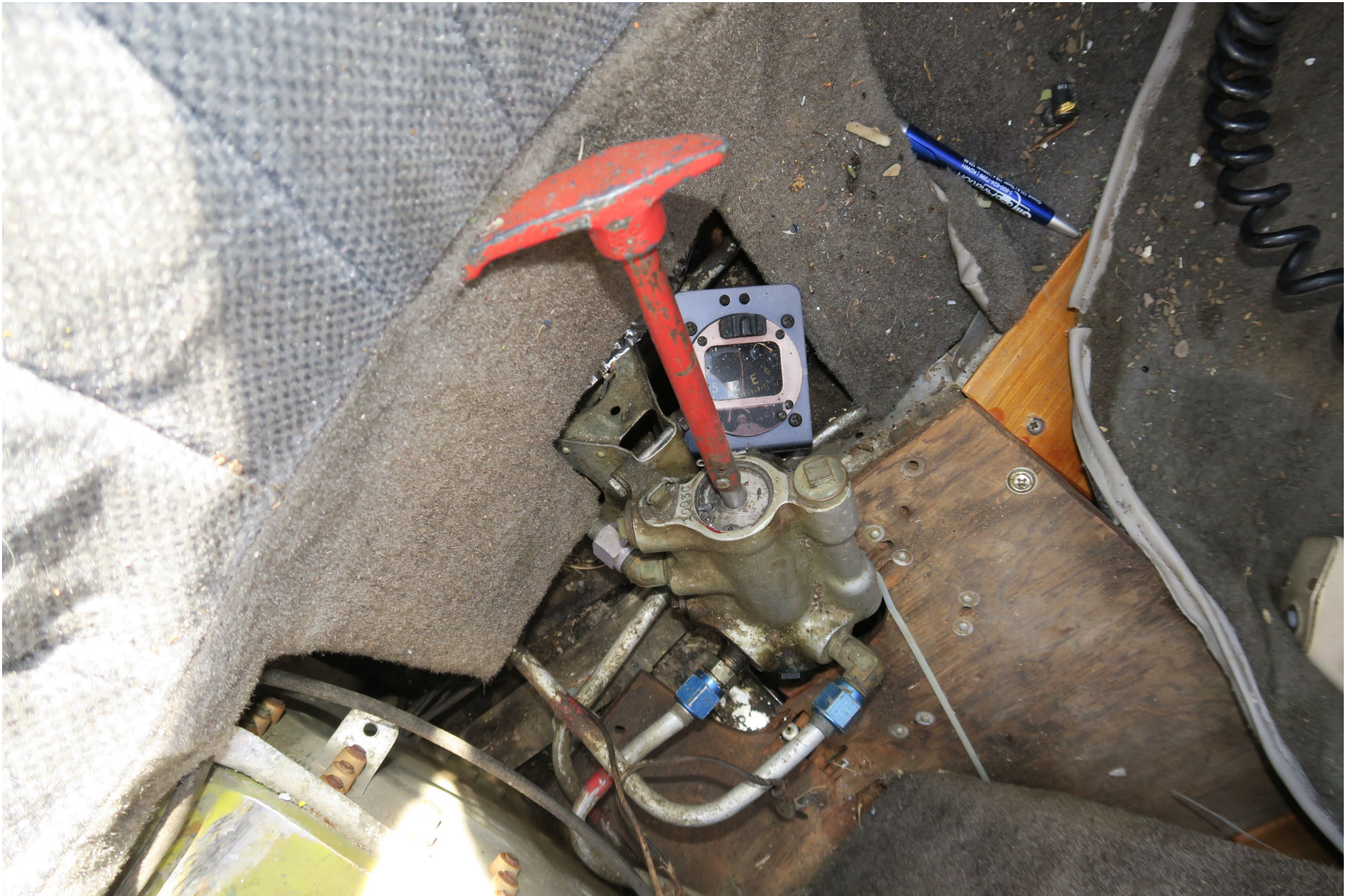
Photo 5 – View of the fuel selector in the cockpit (courtesy of Textron Aviation).
