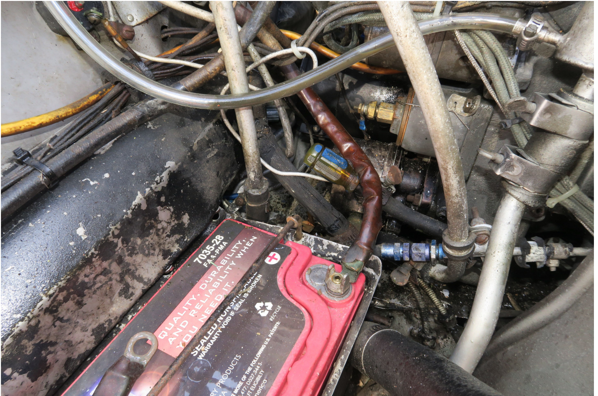
Photo 12 – View of the engine compartment, with a screwdriver plugging a rubber hose (courtesy of Textron Aviation).
