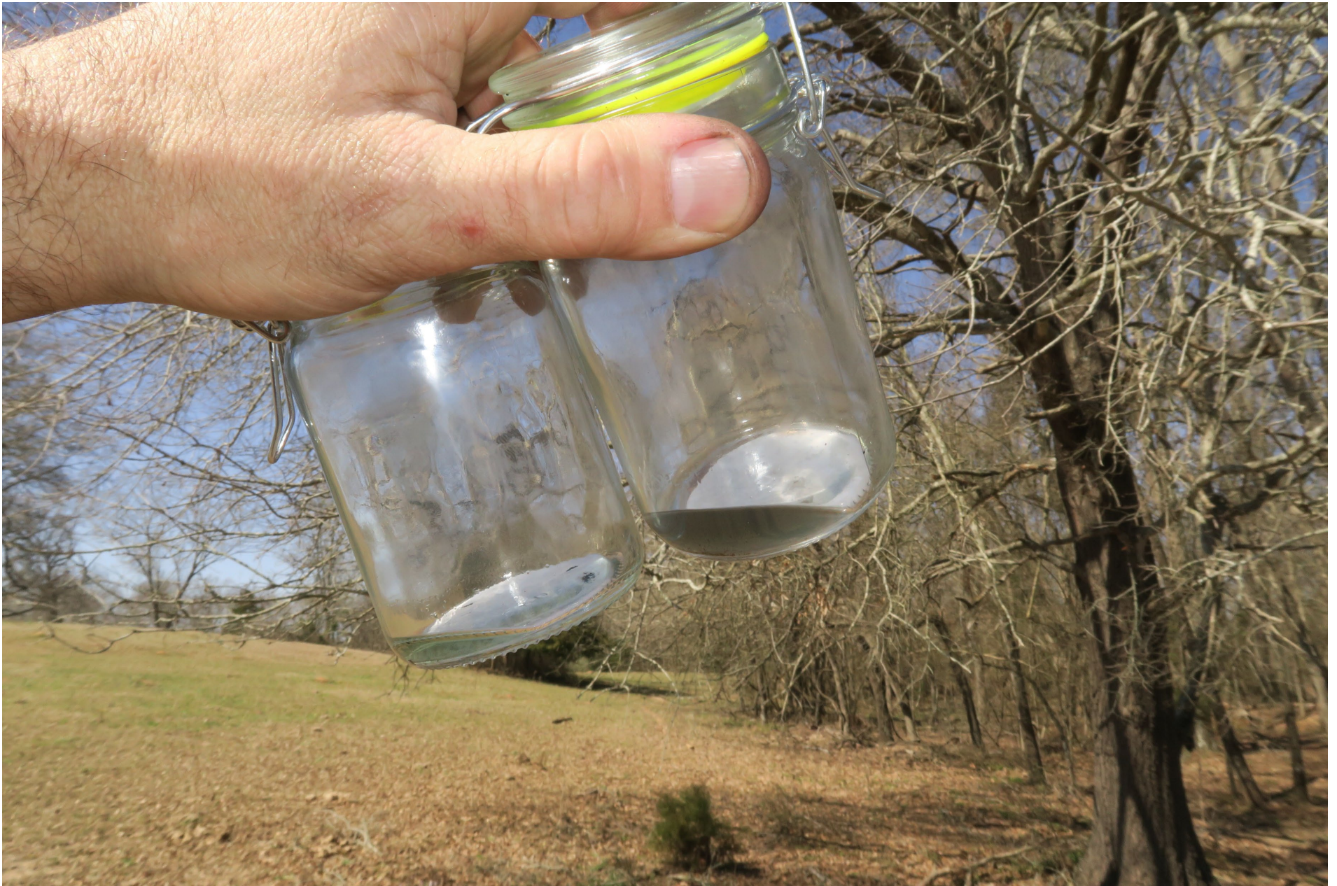
Photo 7 – View of the total amount of fuel obtained from the fuel selector (courtesy of Textron Aviation).
