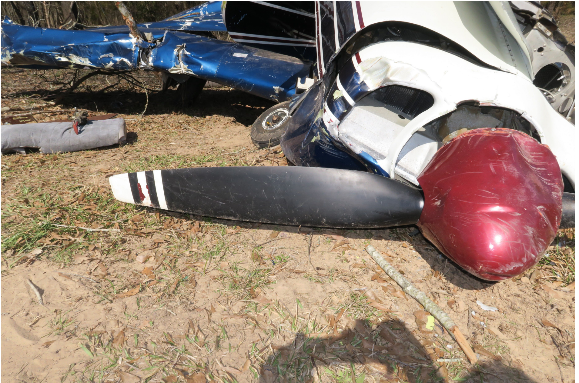
Photo 10 – View of a propeller blade, on the right side of the airplane, at the accident site (courtesy of Textron Aviation).
