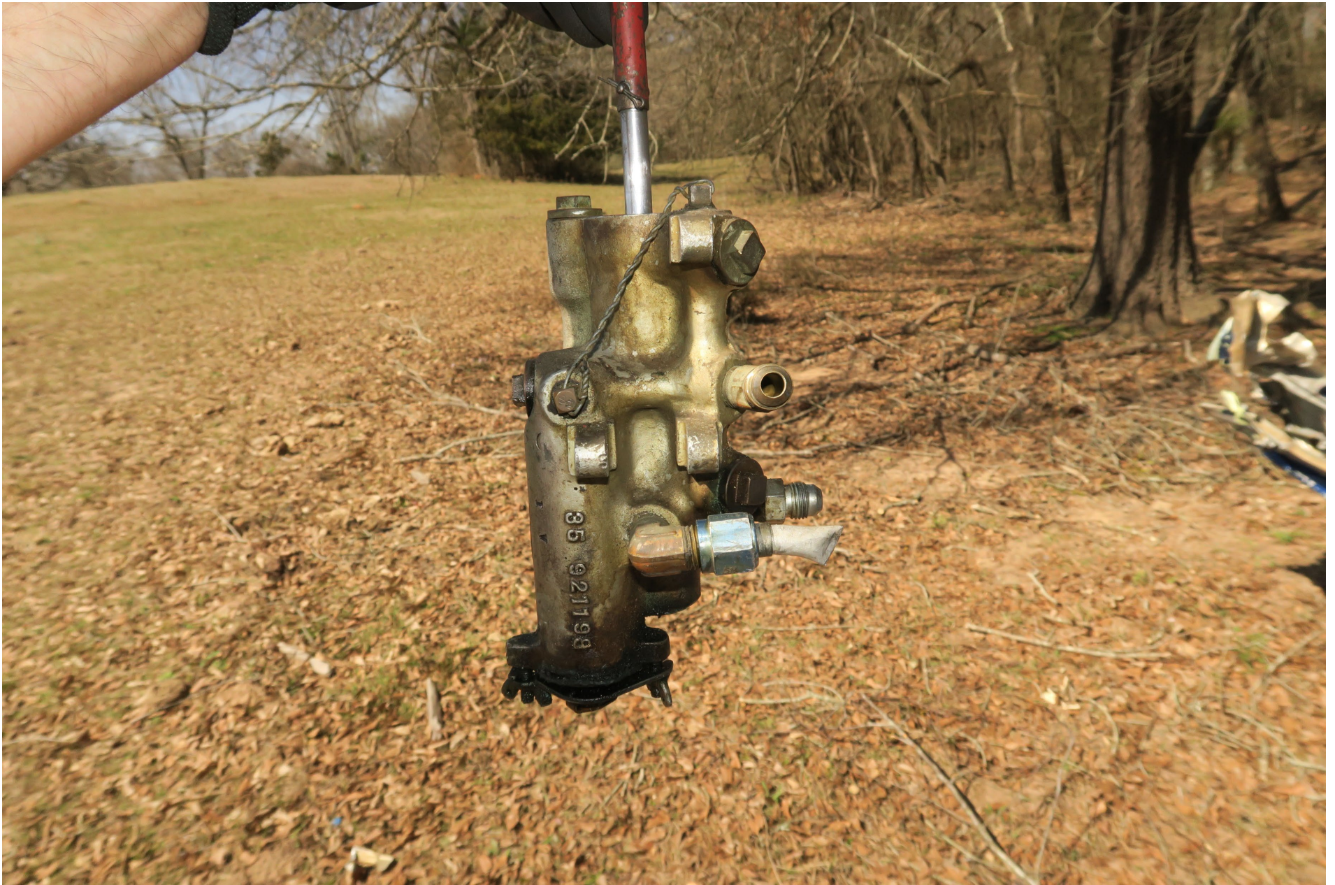
Photo 6 – View of the fuel selector removed from the airplane (courtesy of Textron Aviation).
