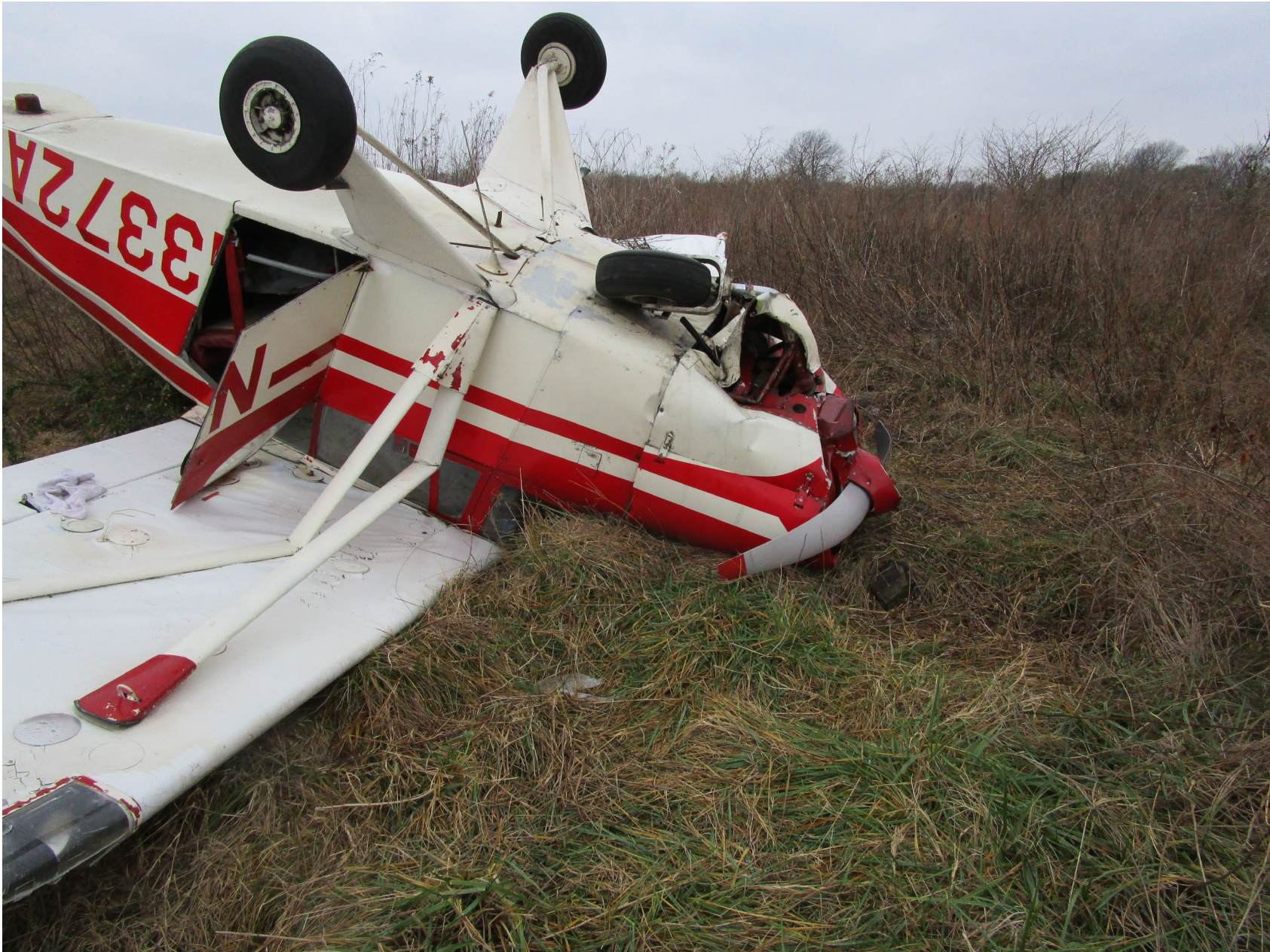
Photo 1 – View of the substantial damage sustained to the left-wing lift struts (courtesy of the Federal Aviation Administration).
