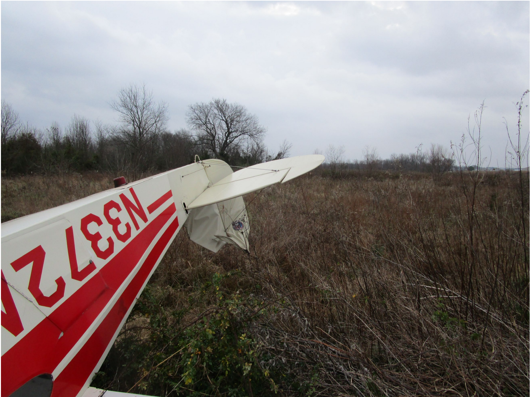
Photo 2 – View of the substantial damage sustained to the vertical stabilizer and the rudder (courtesy of the Federal Aviation Administration).
