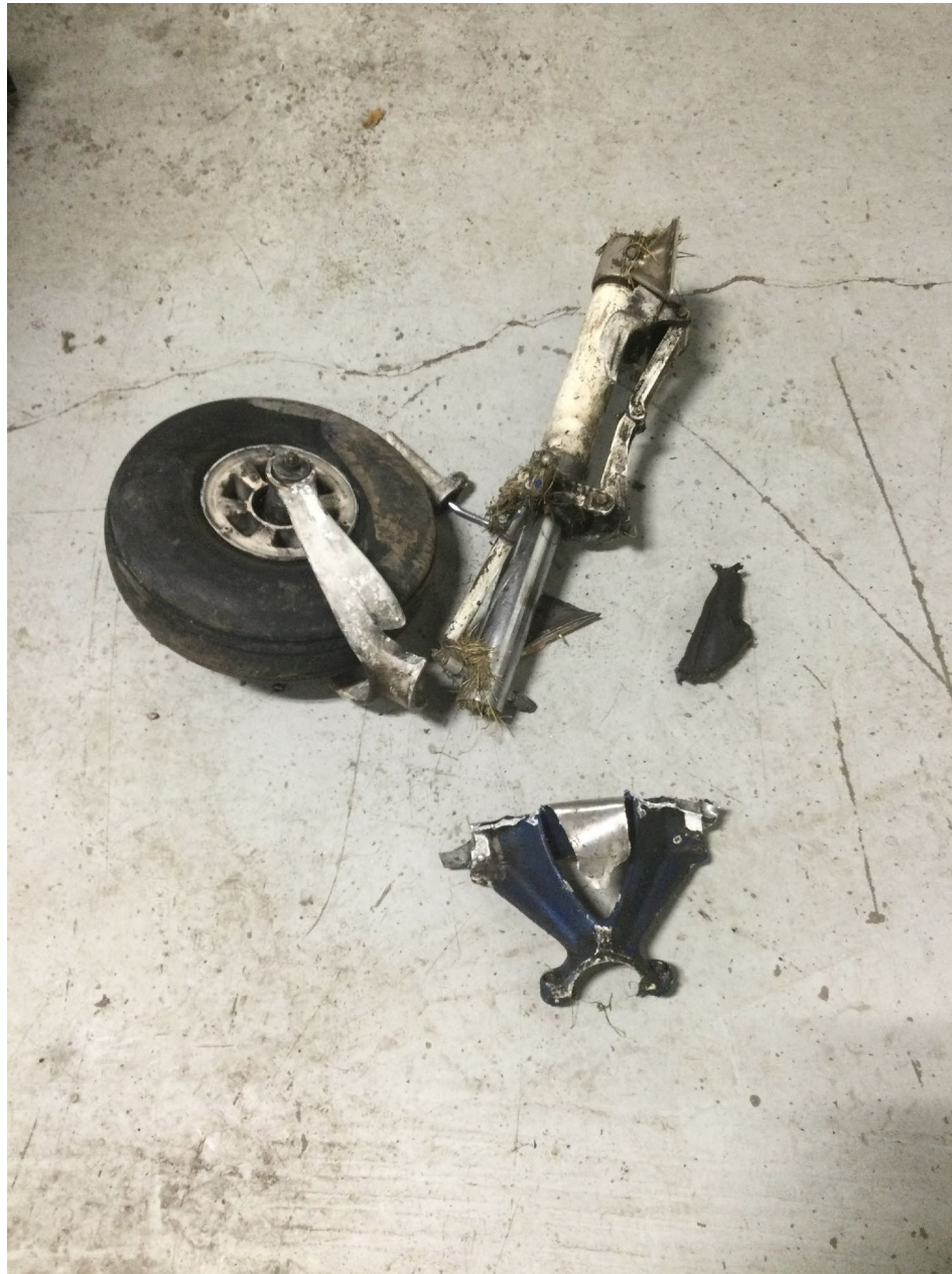
Photo 2 – Close-up view of the separated nose wheel assembly (courtesy of the Federal Aviation Administration).
