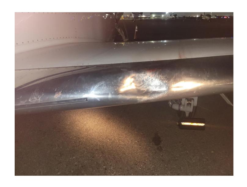
**Photo 1 – Damage to Inboard Left Wing Leading Edge (Courtesy of Operator)**
