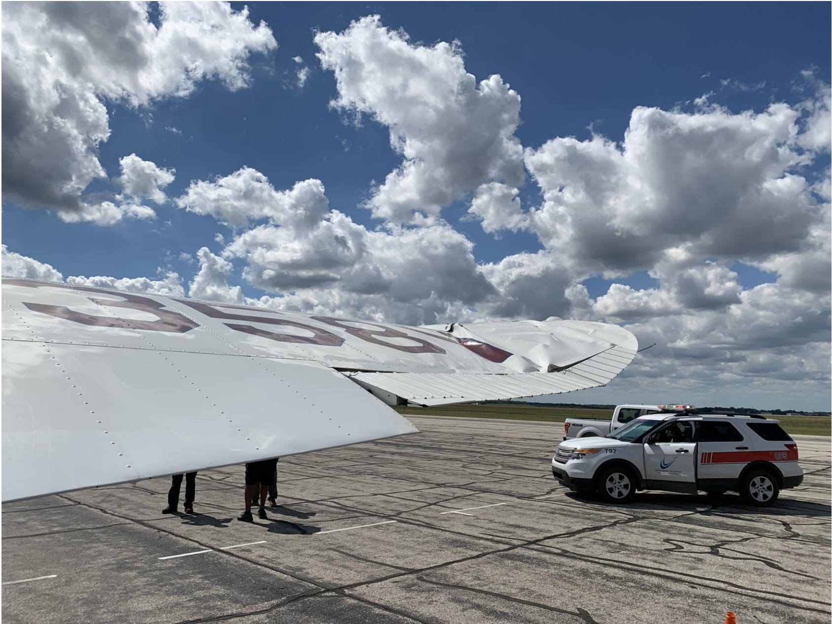
Photo 2 – Rear view of the substantial damage sustained to the right wing (courtesy of the Federal Aviation Administration).
