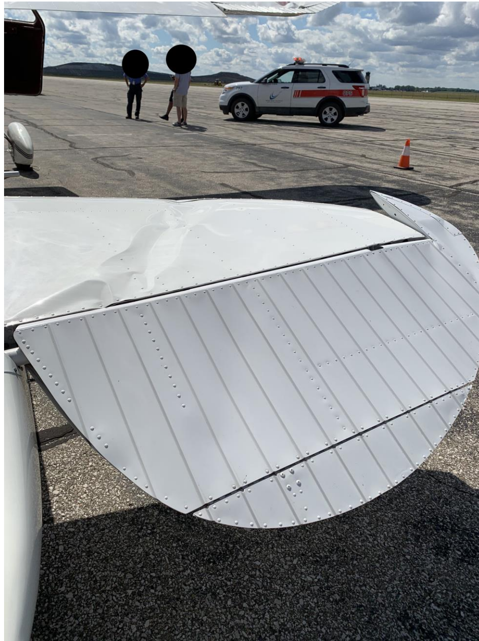
Photo 3 – Rear view of the substantial damage sustained to the right horizontal stabilizer (courtesy of the Federal Aviation Administration).
