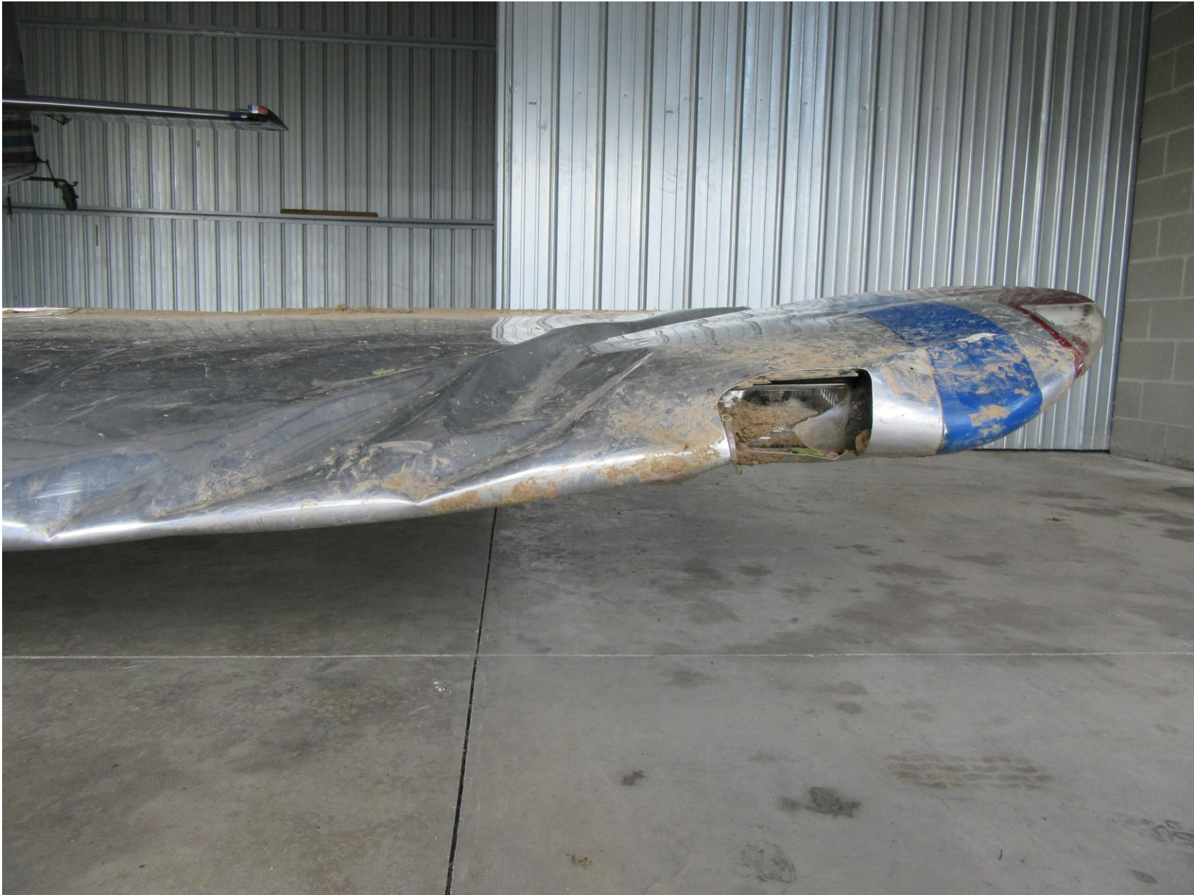
Photo 4 – Close up view of the substantial damage sustained to the left wing (courtesy of the Federal Aviation Administration).
