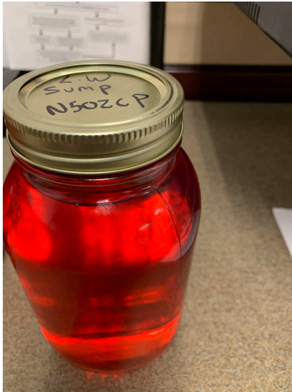
Photo 8 – View of a glass fuel sample jar, with a sample obtained from the left wing sump (courtesy of the Federal Aviation Administration).
