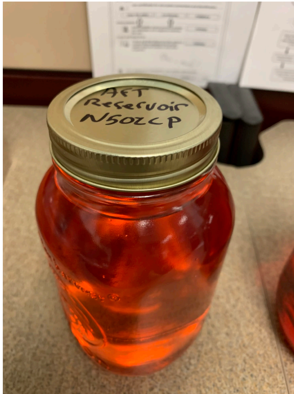
Photo 12 – View of a glass fuel sample jar, with a sample obtained from the aft reservoir (courtesy of the Federal Aviation Administration).
