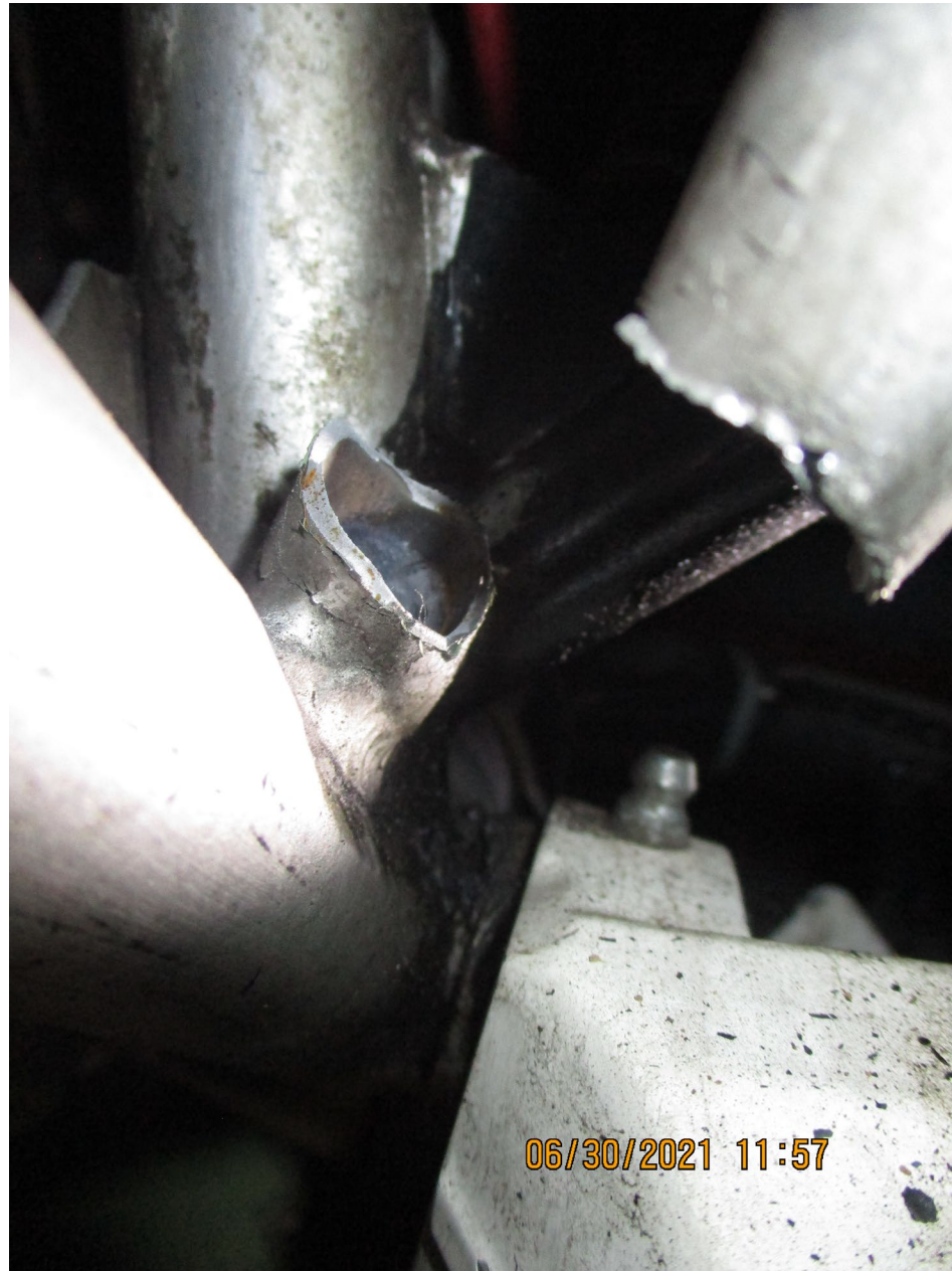
Photo 7 – Close up view of the fracture sustained to the lower portion of the engine mount (courtesy of the Federal Aviation Administration).
