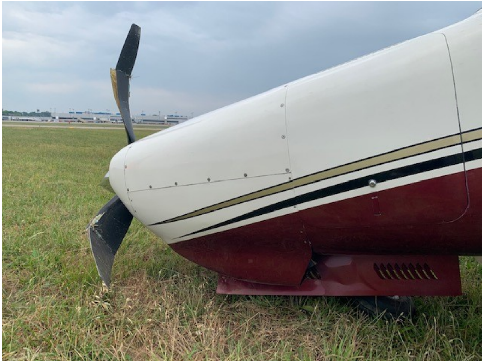
Photo 4 – Close up left side view of the collapsed nose landing gear at the accident site (courtesy of the Federal Aviation Administration).
