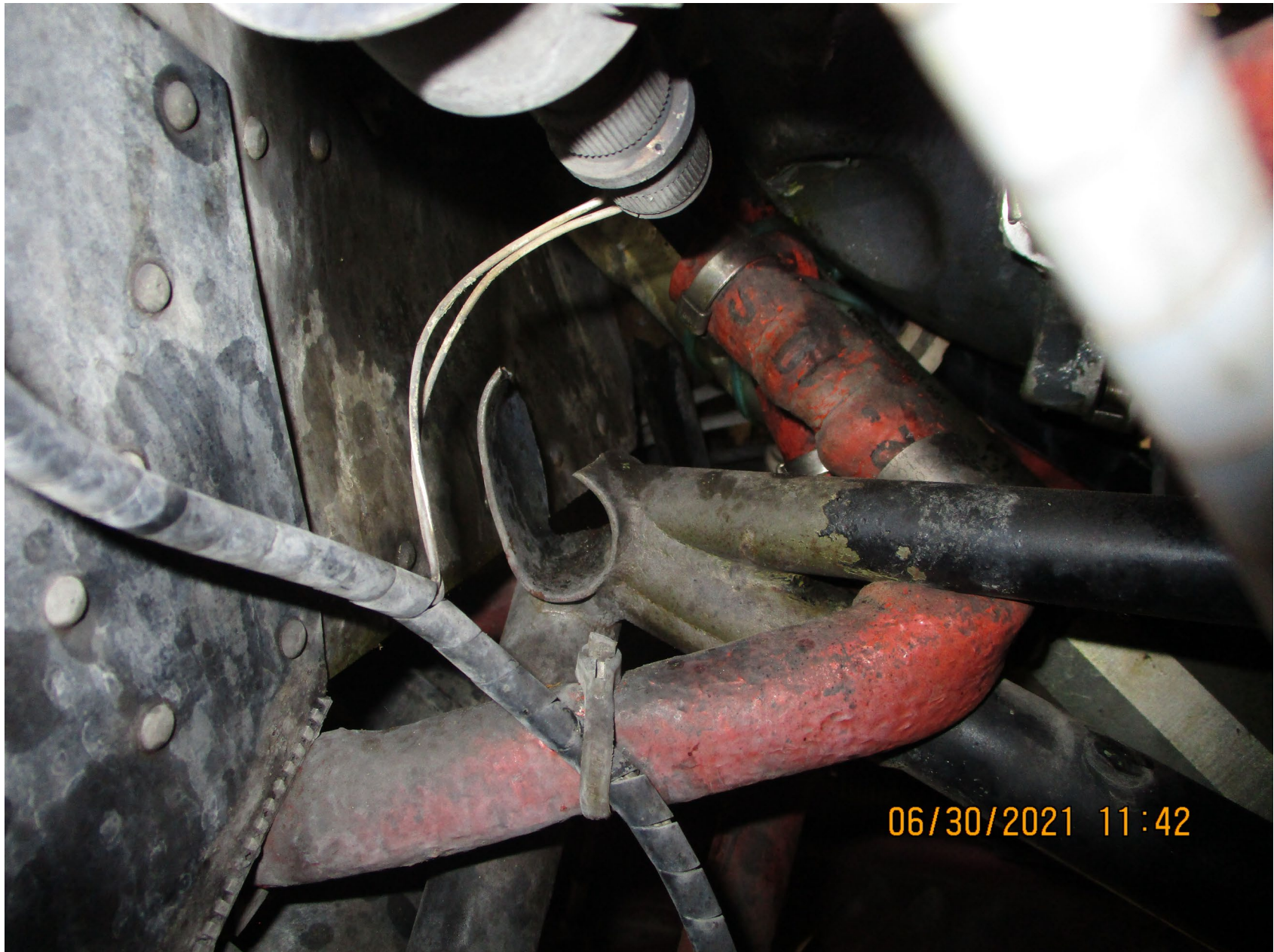
Photo 5 – Close up view of the fracture sustained to the upper portion of the engine mount (courtesy of the Federal Aviation Administration).
