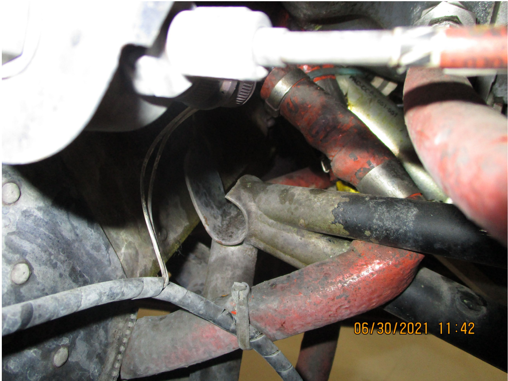
Photo 6 – Close up view of the fracture sustained to the upper portion of the engine mount (courtesy of the Federal Aviation Administration).
