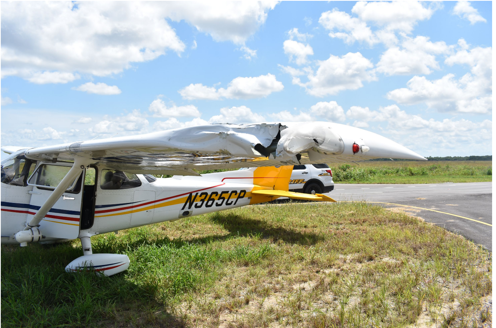
Photo 2 – View of the substantial damage sustained to the left wing (courtesy of the Federal Aviation Administration).
