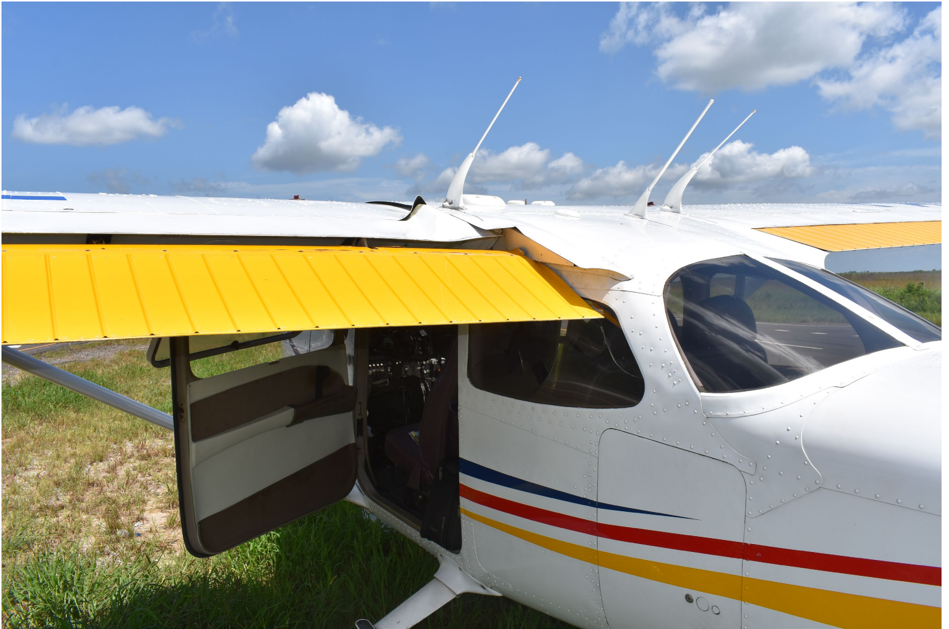
Photo 4 – View of the substantial damage sustained to the left wing (courtesy of the Federal Aviation Administration).
