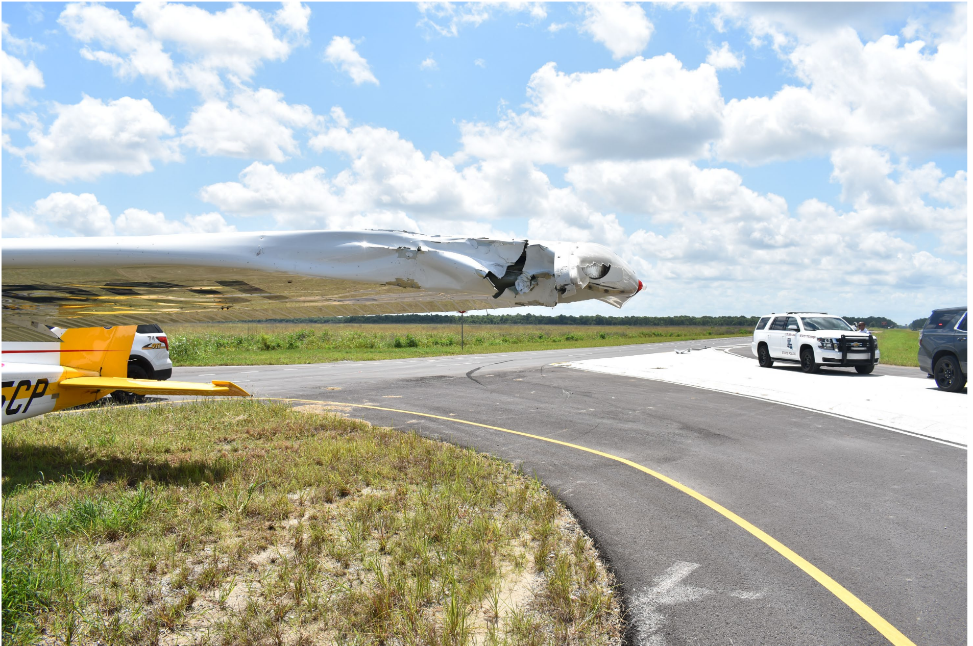
Photo 3 – View of the substantial damage sustained to the left wing and of the road used during the emergency landing (courtesy of the Federal Aviation Administration).
