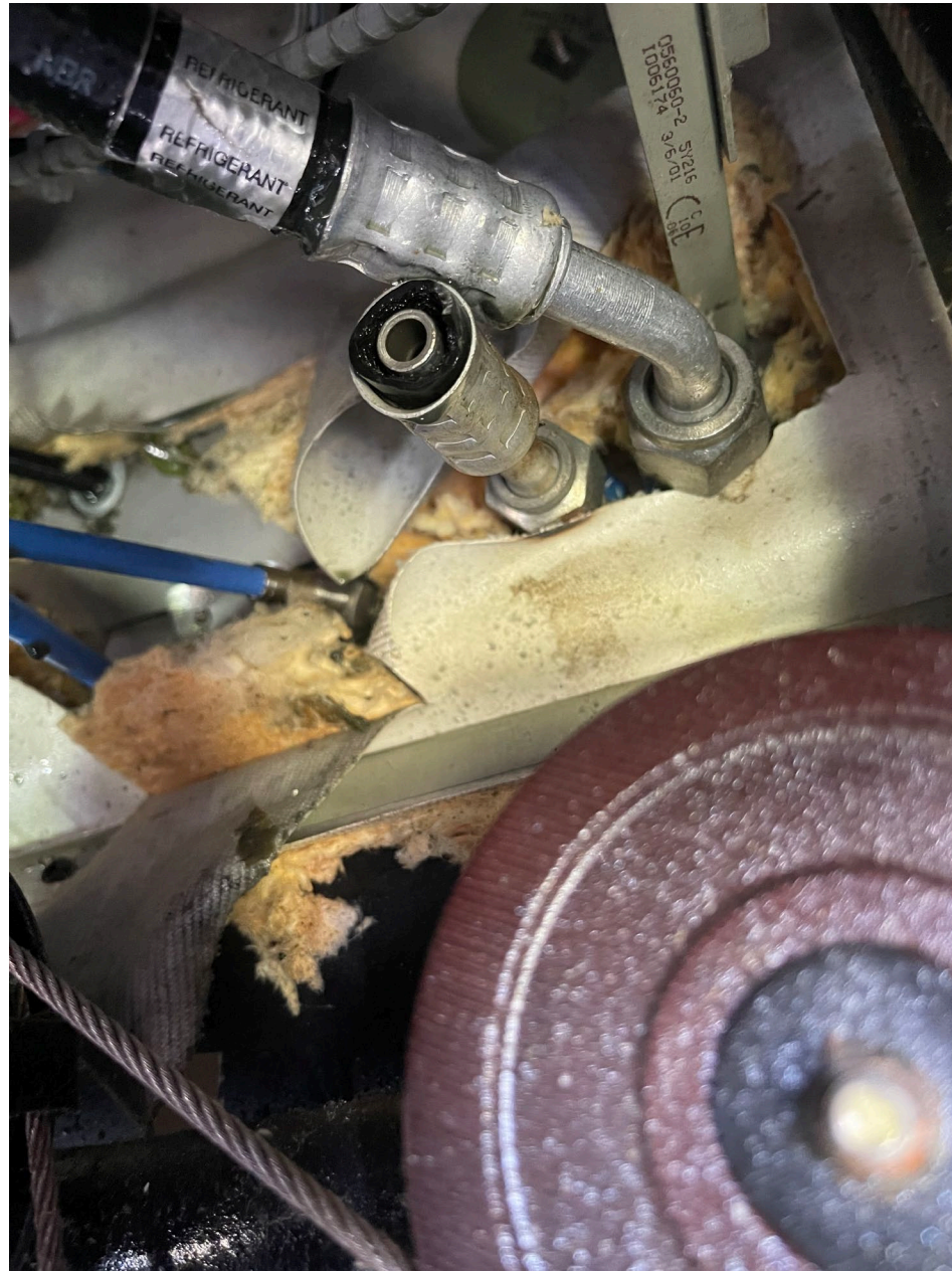
Photo 5 – View of the rubber air conditioning hose that failed at the metal crimp connection (courtesy of the Federal Aviation Administration).
