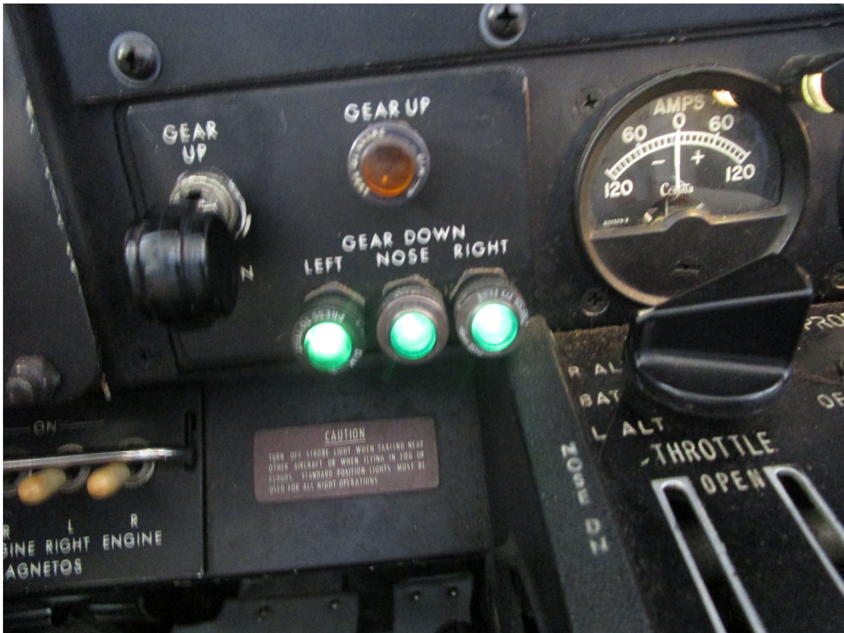
Photo 5 – Close up view of the cockpit-based main landing gear lever and status indicator lights (courtesy of the Federal Aviation Administration).
