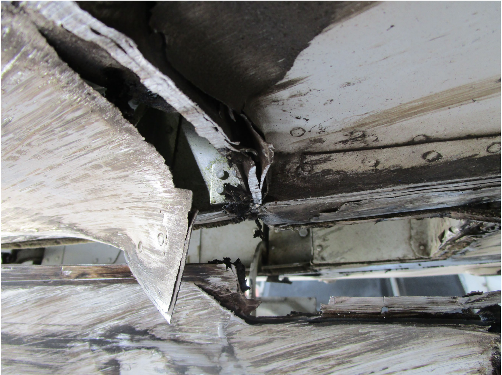
Photo 4 – Close up view of the substantial damage sustained to the bottom of the fuselage (courtesy of the Federal Aviation Administration).
