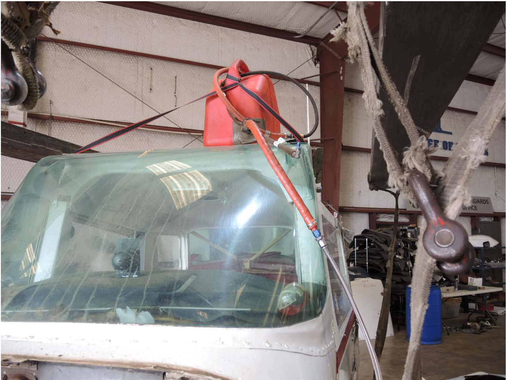
Photo 5 – Front view of the installed fuel tank to facilitate the engine run (courtesy of the National Transportation Safety Board).
