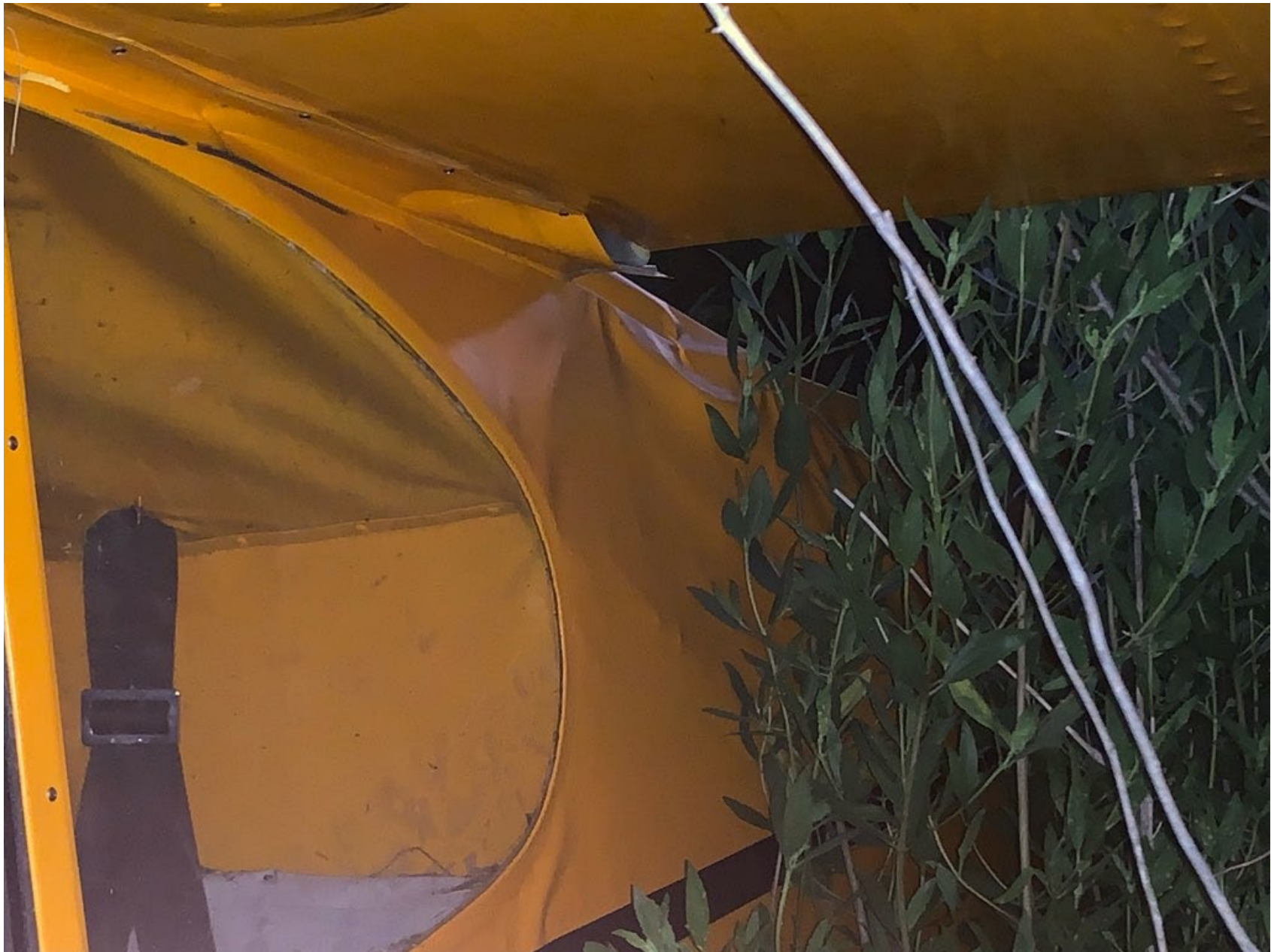
Photo 1 – Substantial Damage to Fuselage (photograph provided by the pilot/owner)
