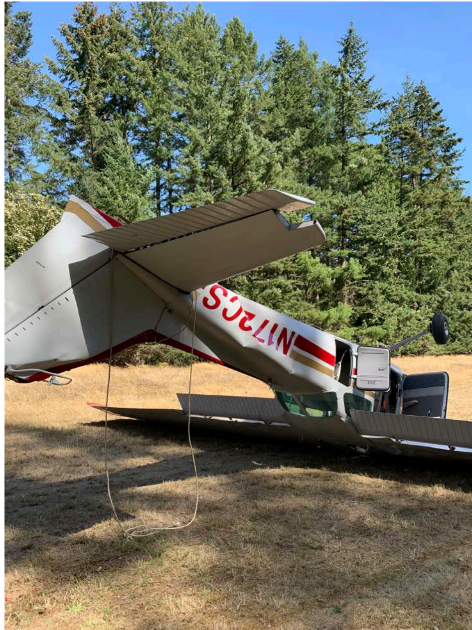
Photo 2 – View of nosed over airplane with damaged tailcone (courtesy of the pilot)
