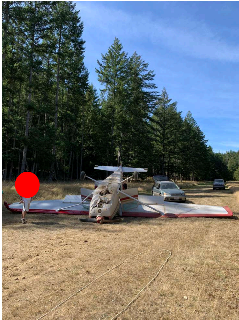
Photo 1 – View of nosed over airplane with a damaged left-wing lift strut (courtesy of the pilot)
