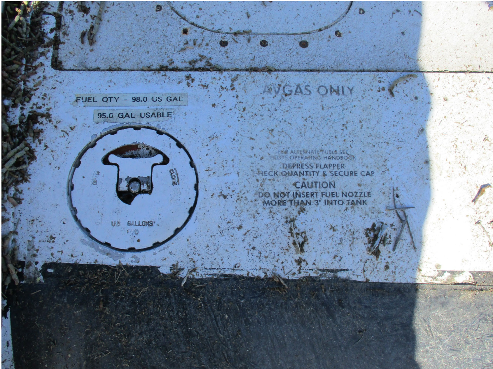
Photo 2 – View of secured gas cap with AVGAS ONLY sticker (courtesy of local law enforcement)
