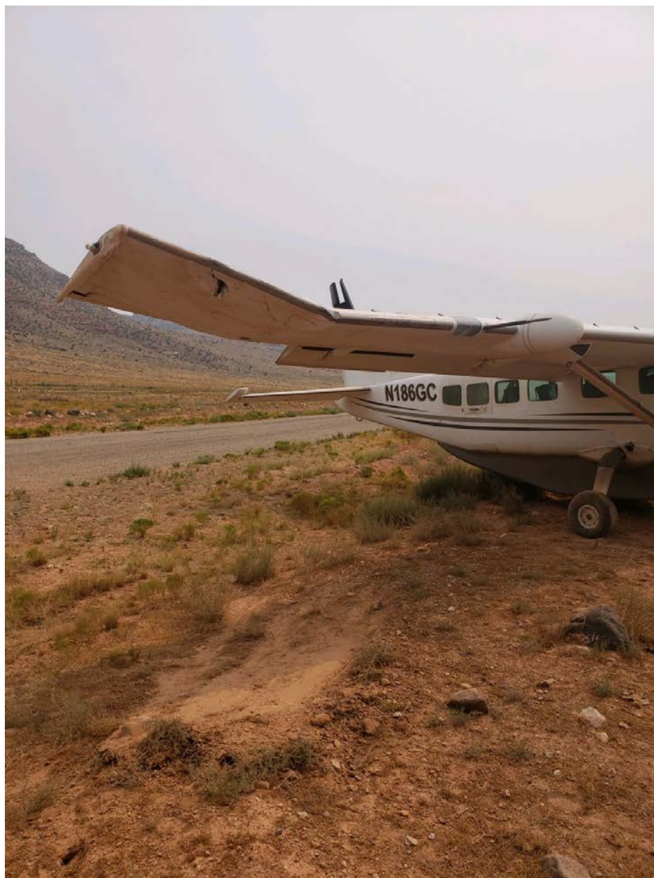
Photo 1 – View of damaged right wing (courtesy of operator)
