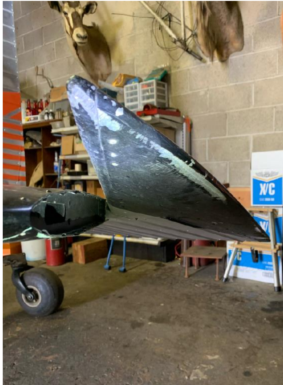
Photo 2 – View of damage to left elevator (photo courtesy of the pilot)
