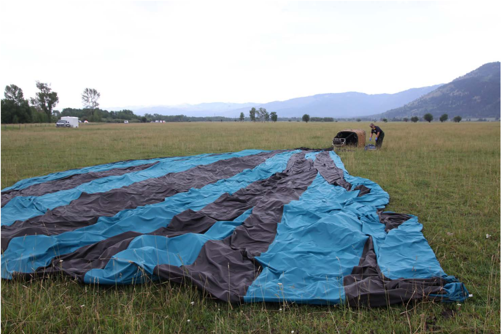
Photo 1 – View of N45303 balloon on its side after impacting terrain (courtesy of local law enforcement officer)
