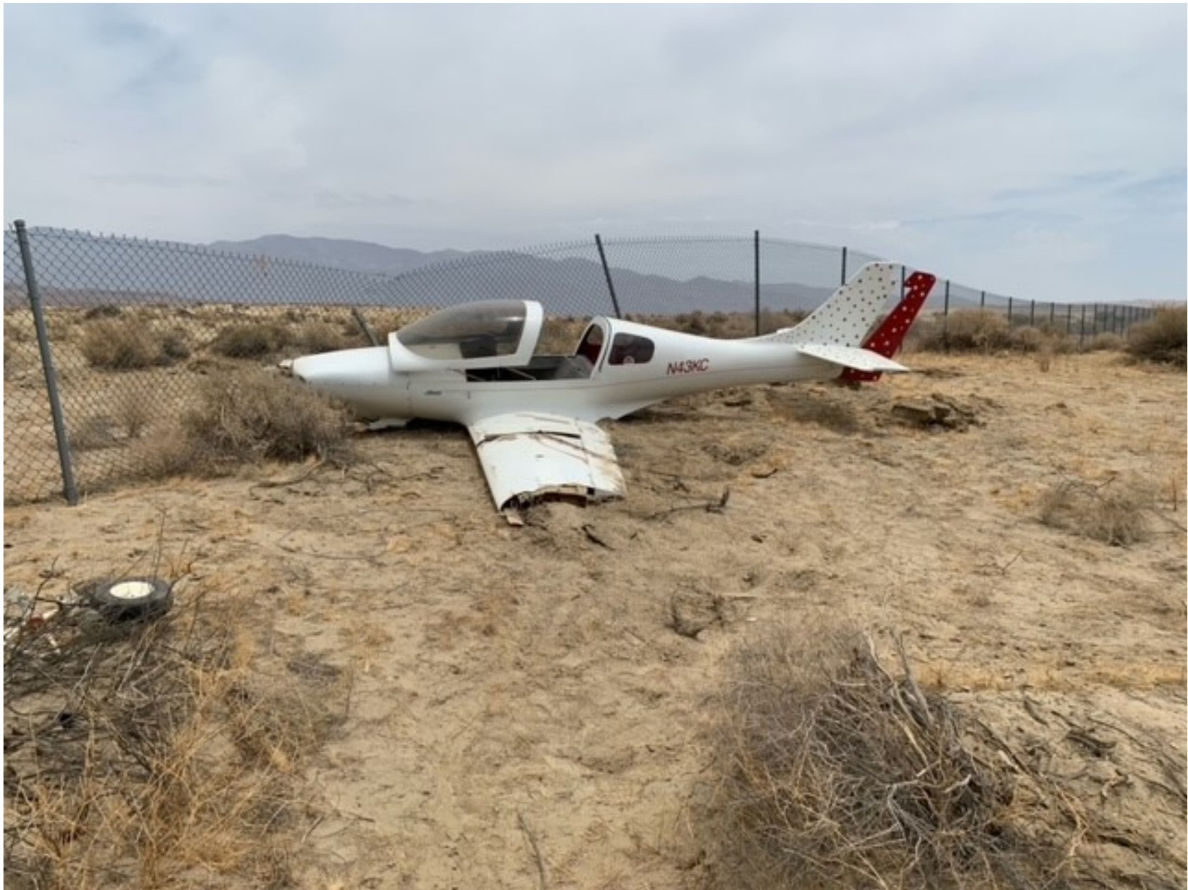
Photo 1 – View of airplane with damaged left wing and rudder (courtesy of the FAA)
