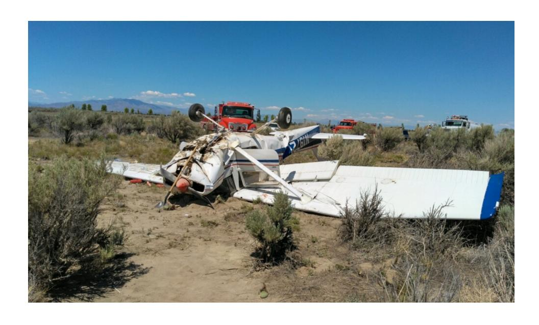
Photo 1 – View of nosed over airplane with damage to fuselage, tailcone, and wings (courtesy of local law enforcement)
