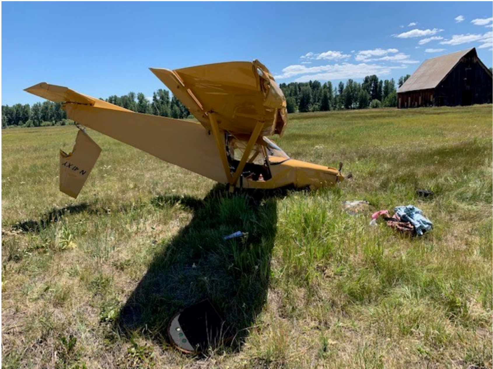
Photo 1 – View of airplane with damaged right wing and rudder (photo courtesy of pilot)
