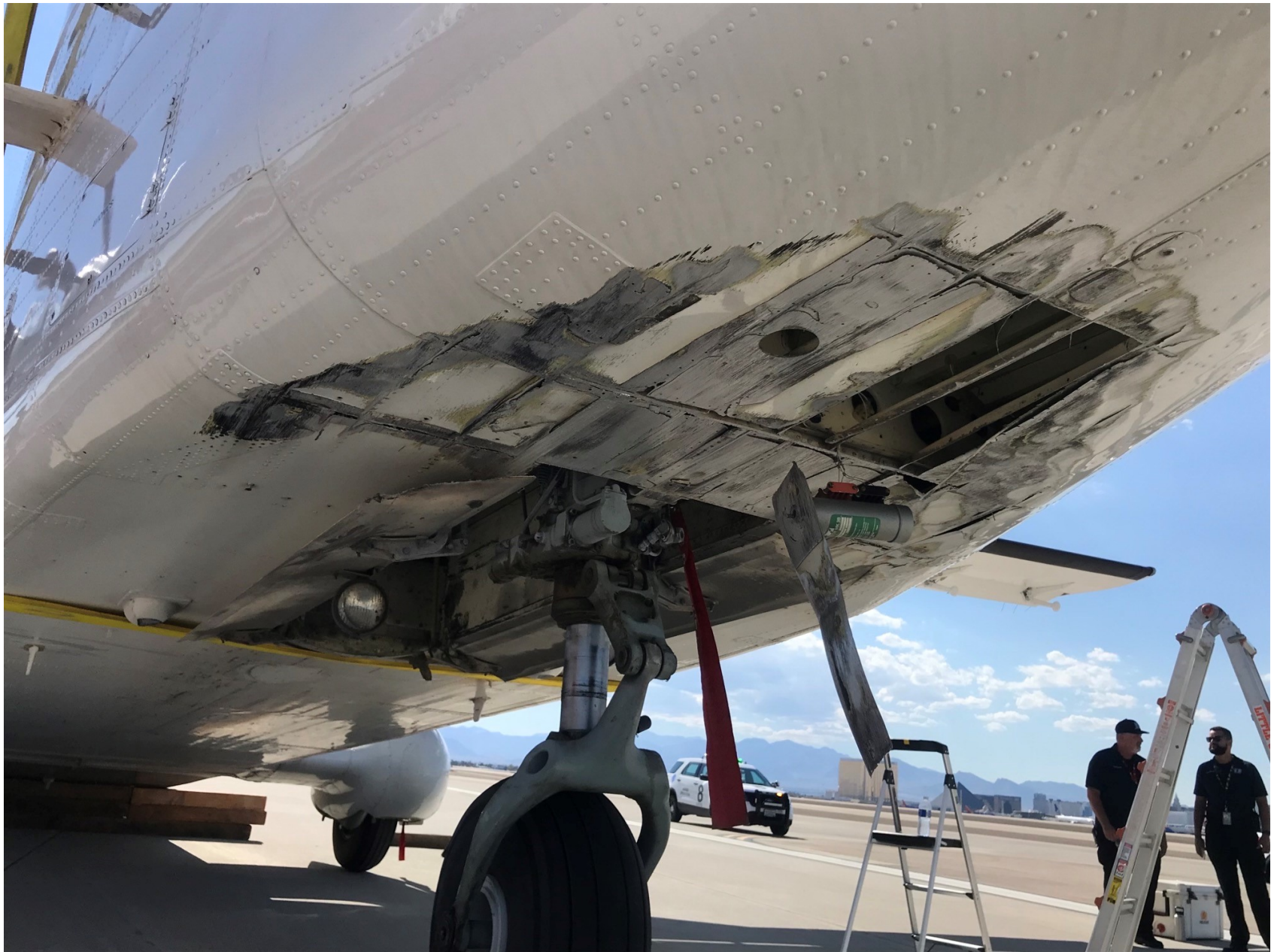
Photo – View of damage to lower fuselage (photo courtesy of the operator)
