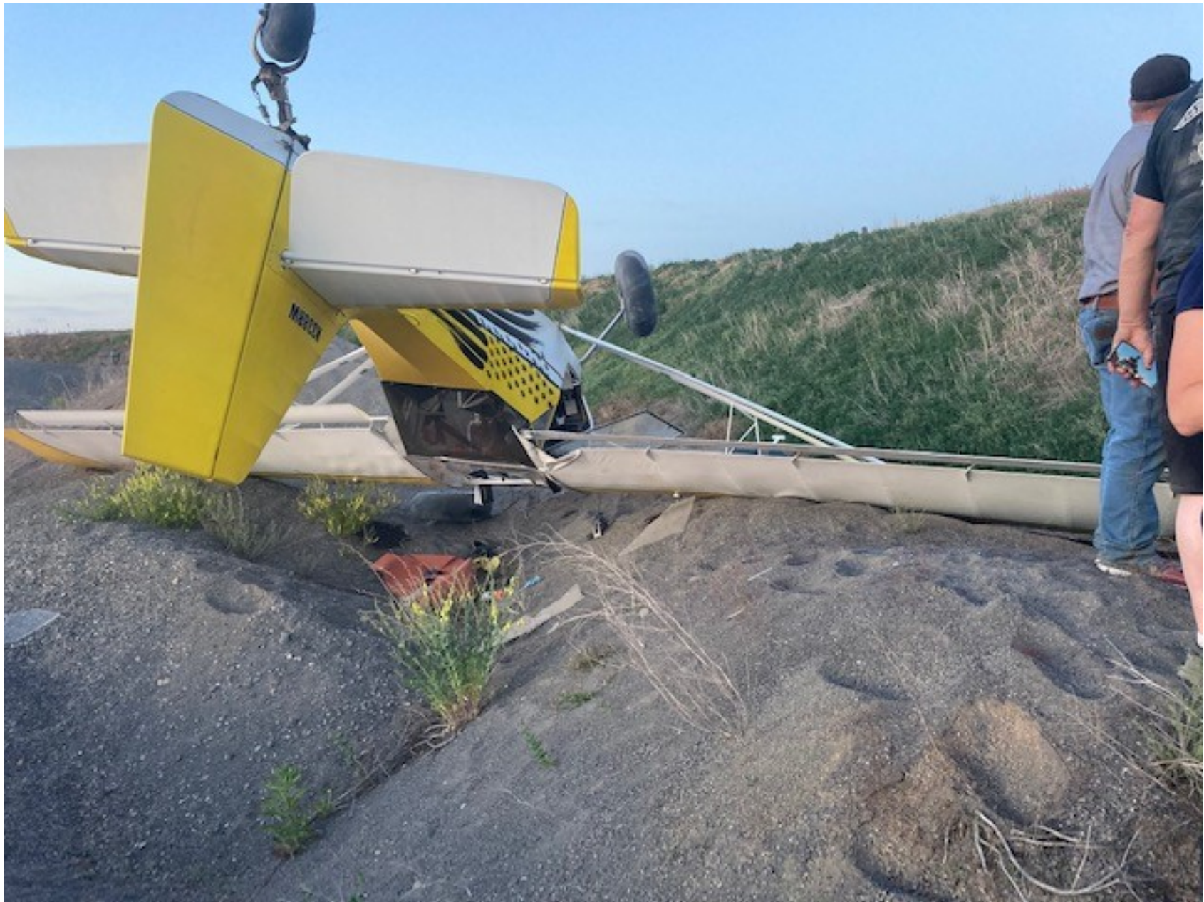
Photo 2 - View of airplane with left wing damage nosed over on a rock quarry (courtesy of the FAA)
