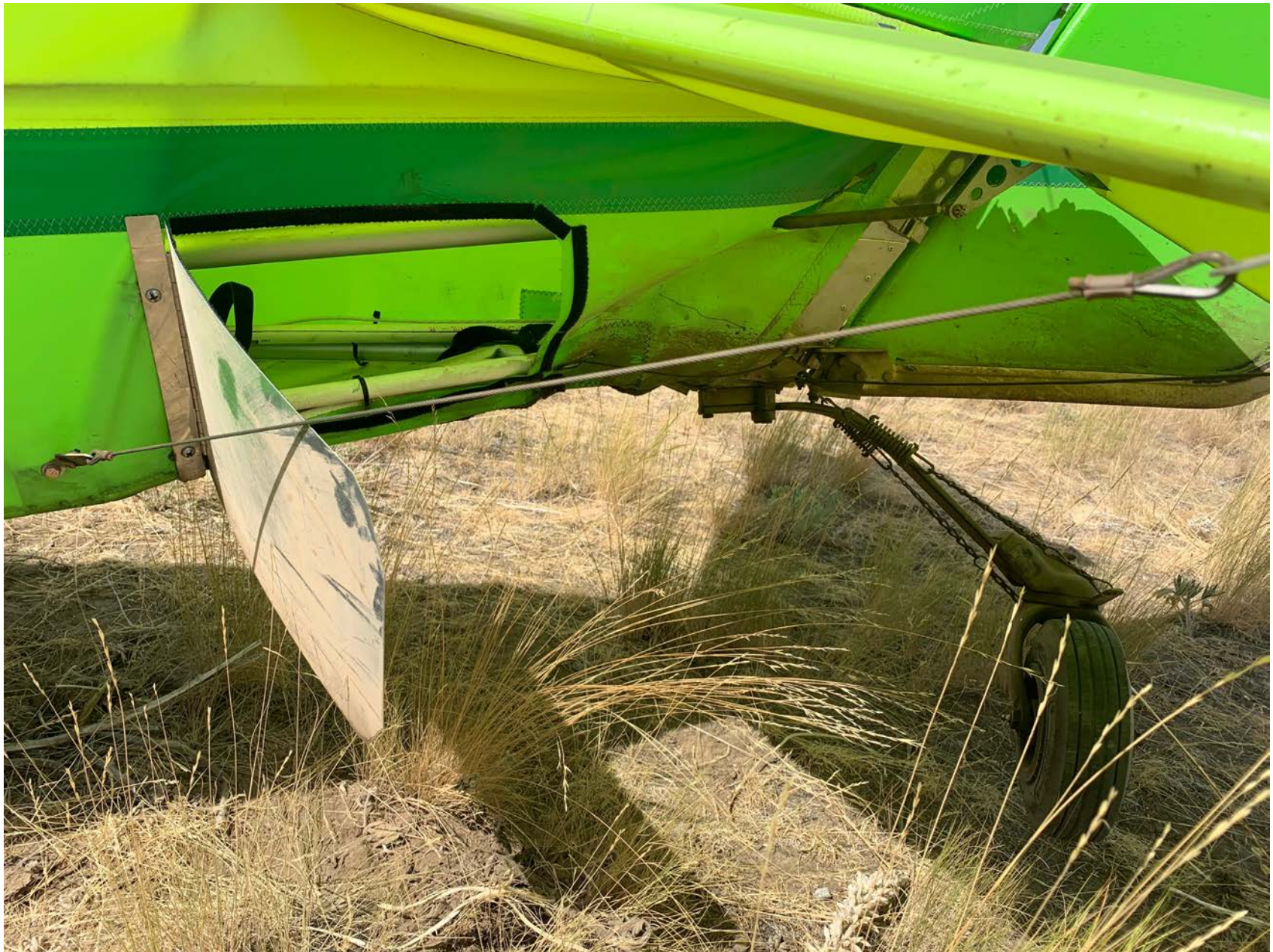
Photo 1 – View of damaged tailcone (courtesy of the FAA)
