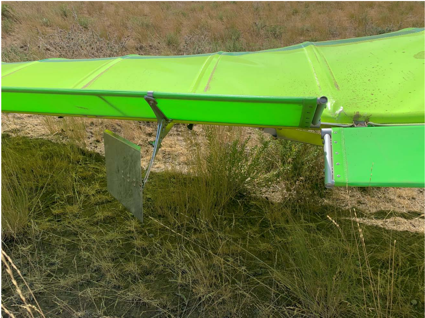
Photo 2 – View of damaged left wing (courtesy of the FAA)
