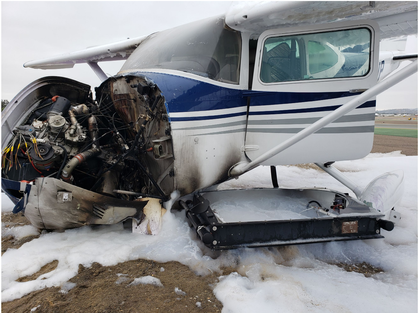
Photo 1 – View of accident airplane with damage to engine truss (courtesy of the FAA)
