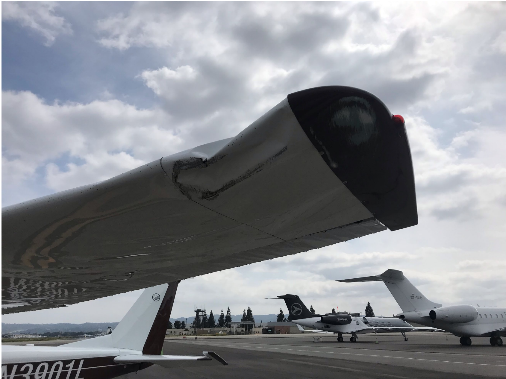
Photo 1 – View of damage to the left wing (photo courtesy of airport operations)
