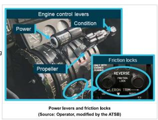
When correctly set, the friction locks provided adequate resistance for the power levers to remain in position. However, if not adequately set, power lever migration could occur. This was typically experienced when the pilot removed their hand from the levers during take-off and could lead to the aircraft yawing towards the engine experiencing the power lever migration, a significant reduction in power, and the auto-feather system disarming.
