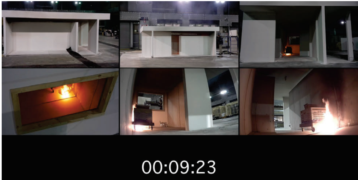
Figure 47: Phase 3, Test 3, Sterno can repositioned at 167 seconds post ignition to ensure that the flame was in contact with plastic ribbing under dolly cart (361119_Master_1345485)
