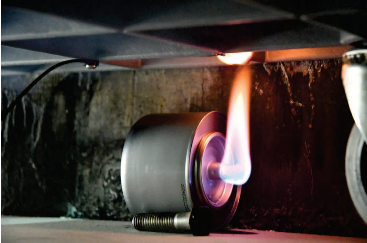
Figure 40: Phase 3, Test 3, Sterno can placement (361119_1339535.JPG)
