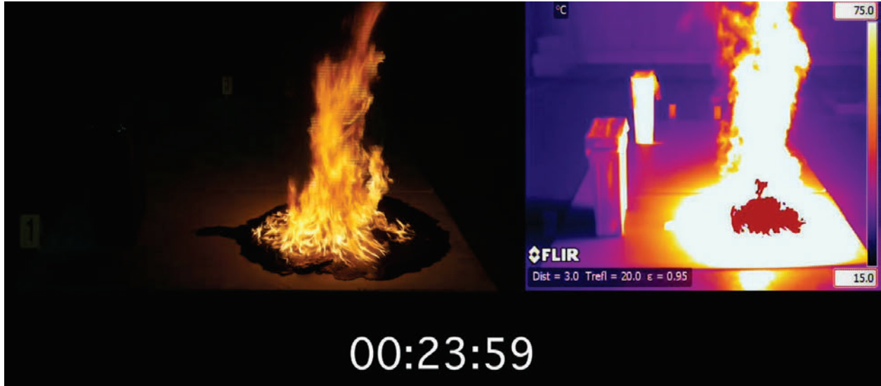
Figure 36: Phase 2, Test 3, Peak burning based on visual observation (361142_Master_1345553) [4]
