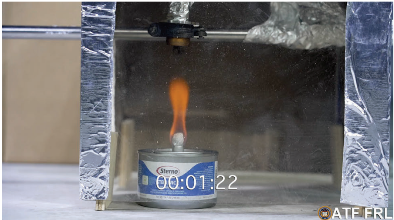
Figure 9: Phase 1, Test 4, Sterno can upright, Screen shot from video (361138_Master_1345552)
