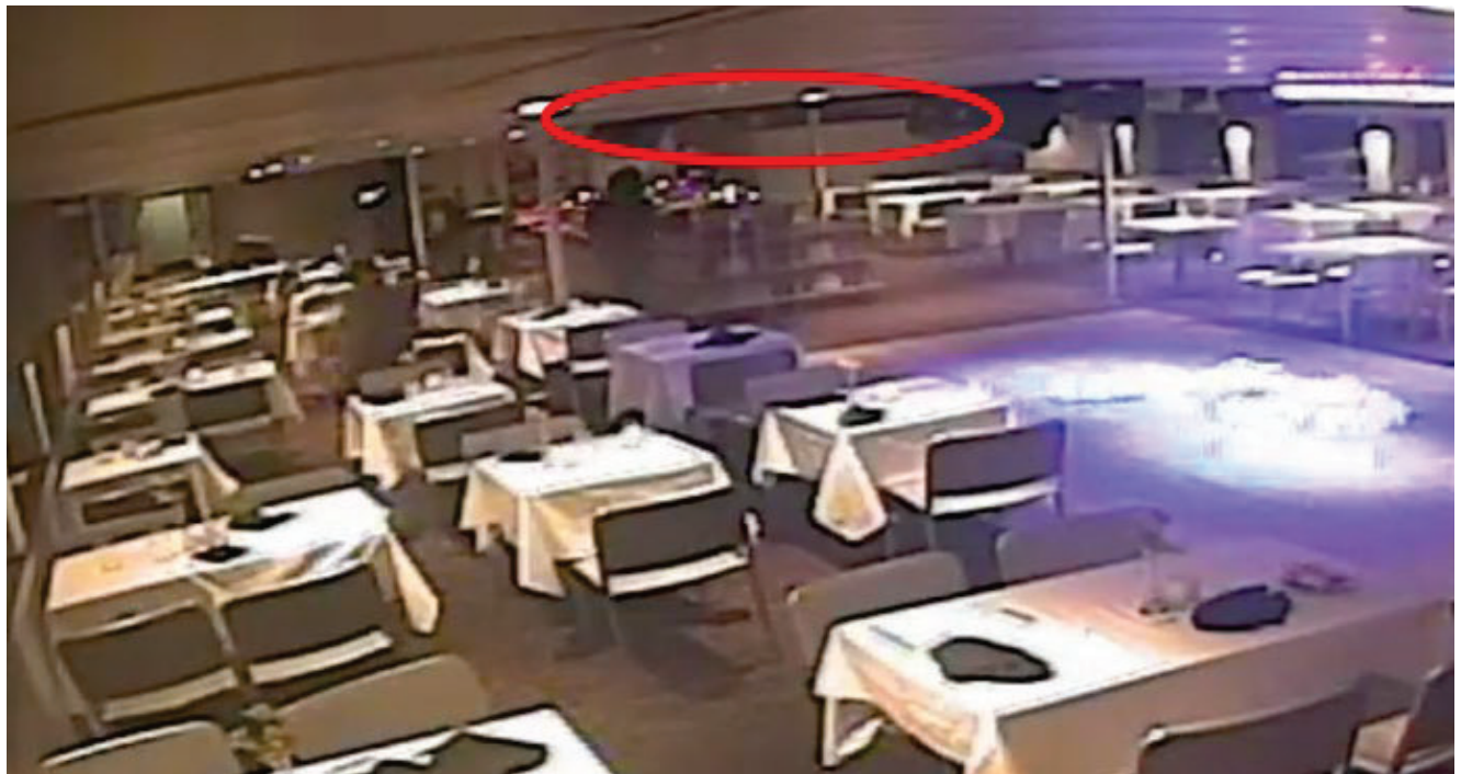
Figure 4: Screenshot of video channel “CH04.h264” from camera aboard the Spirit of Boston prior to fire. Red ellipse marks the location of visible smoke on security camera.
