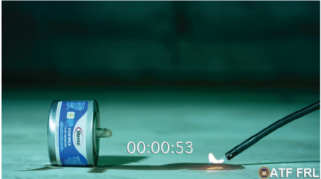
Figure 11: Phase 1, Test 6, Screen shot from video, Attempted ignition of spilled Sterno fuel when can placed on side (361154_Master_1345572)
