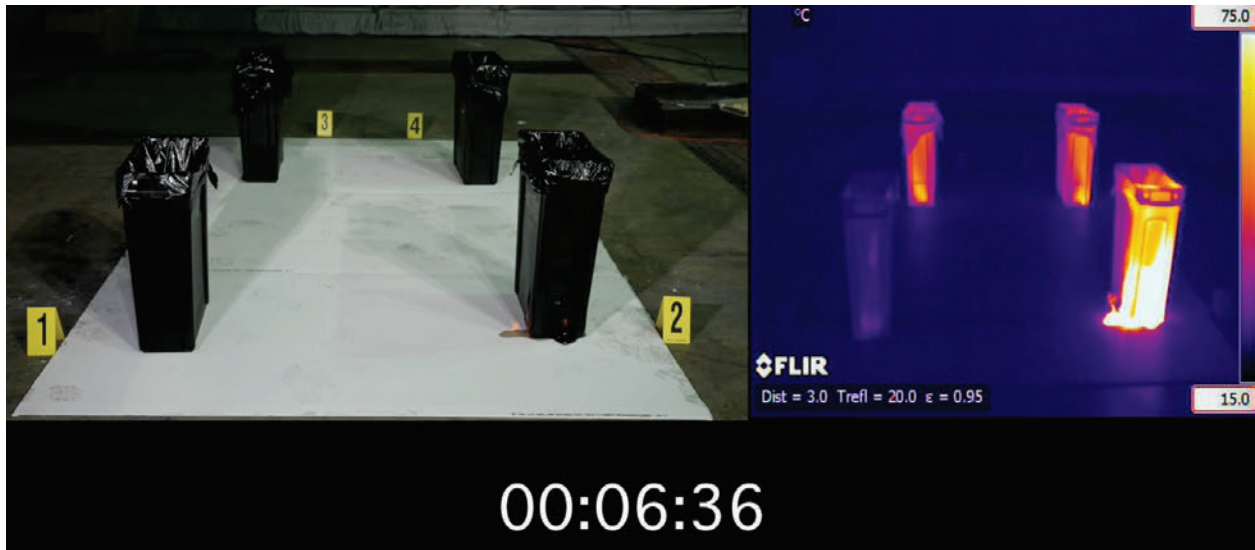
Figure 35: Phase 2, Test 3, Flame outside of trashcan 2 (361142_Master_1345553) [4]
