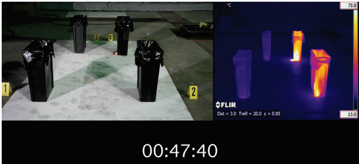
Figure 37: Phase 2, Test 4, Flame outside of trashcan 3 (361155_Master_1345575) [4]
