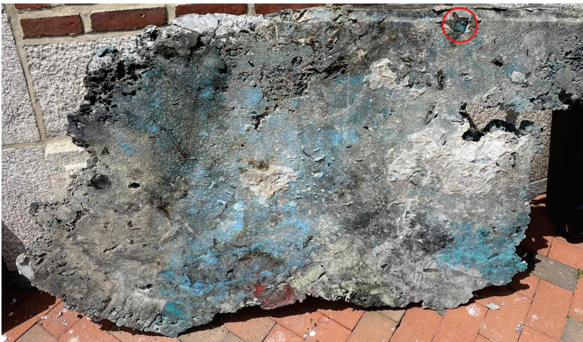
Figure 2: Bottom side of resolidified plastic recovered from room of fire origin, Sterno can resting on its side is circled in red, "Origin 3" cropped, [Photo by SA/CFI H [REDACTED]] (187727_748776.PNG)
