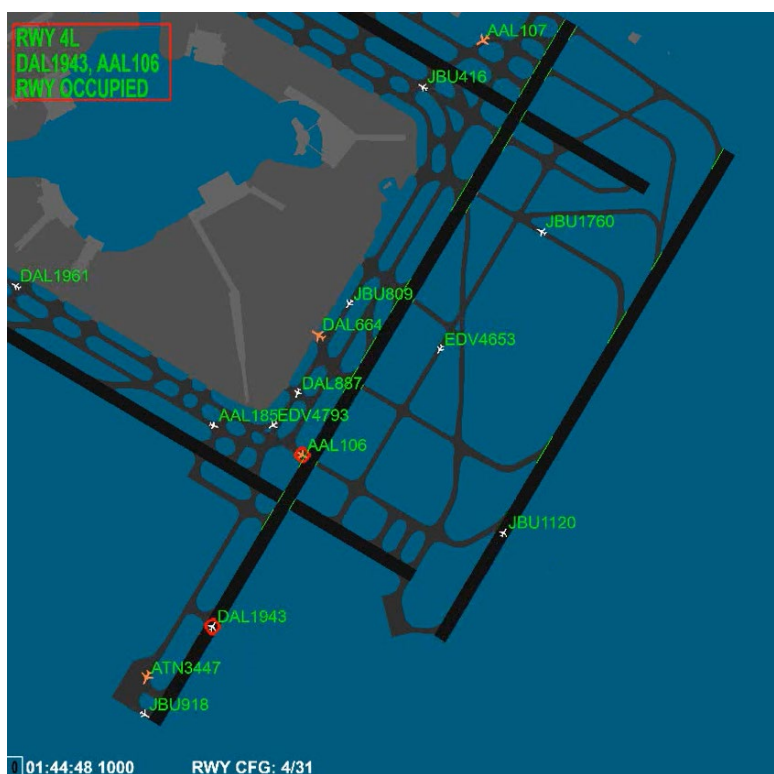
Figure 10. Screen capture of the JFK ASDE-X system display while the runway occupied alert was active for DAL1943 and AAL106.
