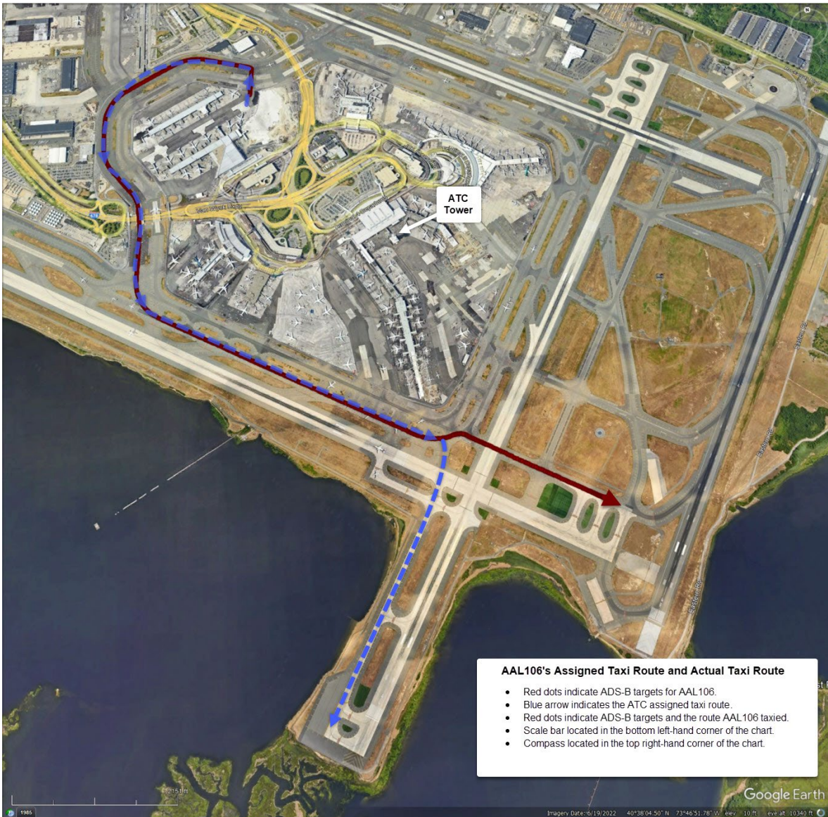
Figure 2. The assigned (blue) and actual (red) taxi routes of AAL106 overlaid on satellite imagery of the JFK airport.
