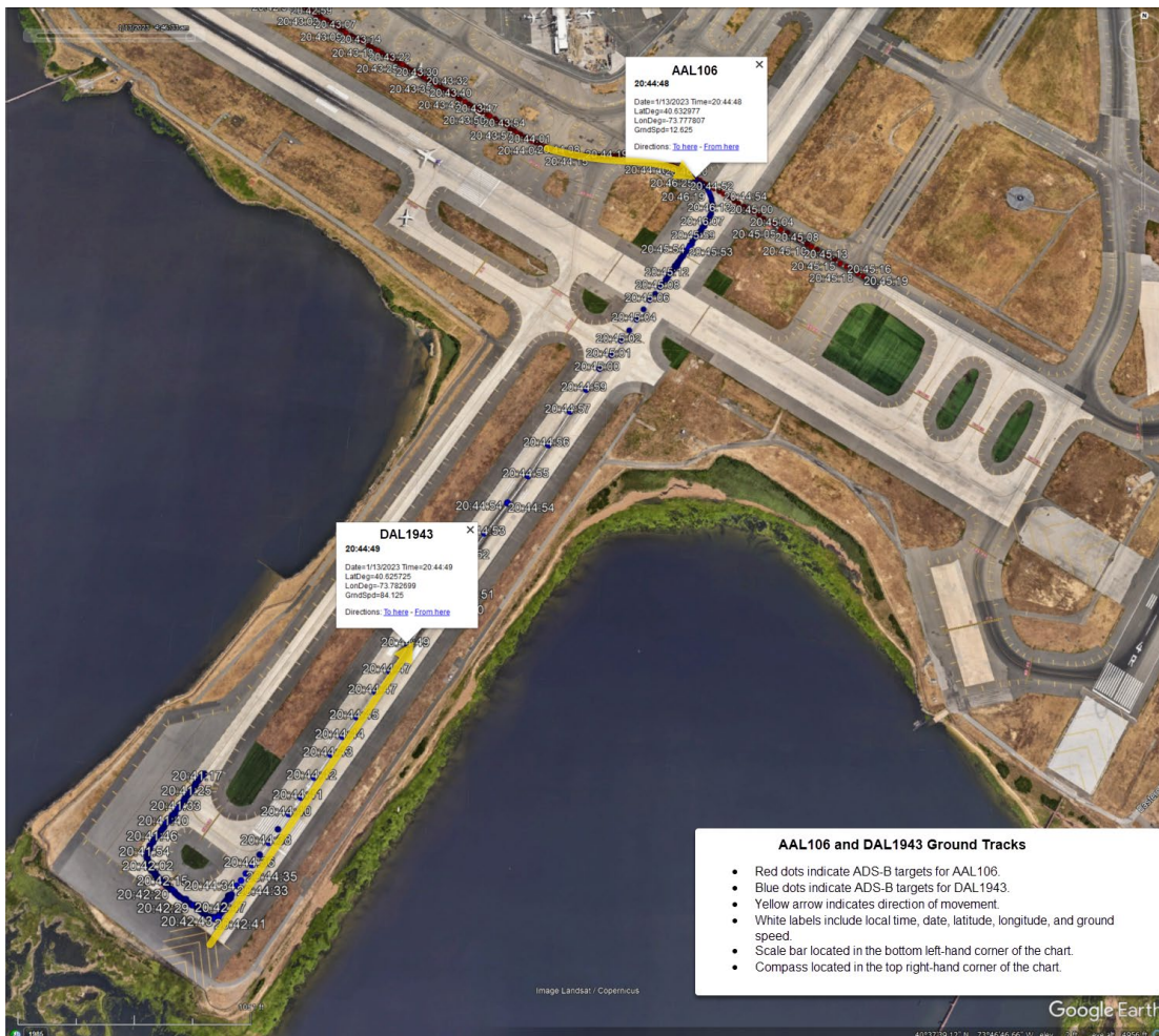
Figure 4. ADS-B ground tracks of AAL106 (red) and DAL1943 (blue) illustrating the location of both airplanes when ATC cancelled the takeoff clearance for DAL1943.
