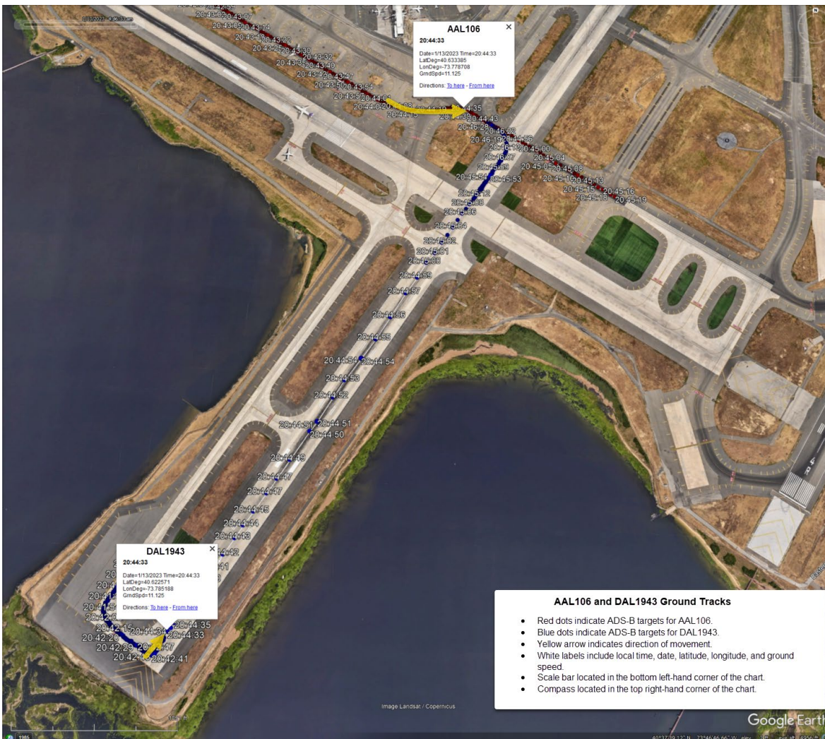
Figure 3. ADS-B ground tracks of AAL106 (red) and DAL1943 (blue) illustrating the location of both airplanes as DAL1943 began their takeoff roll.
