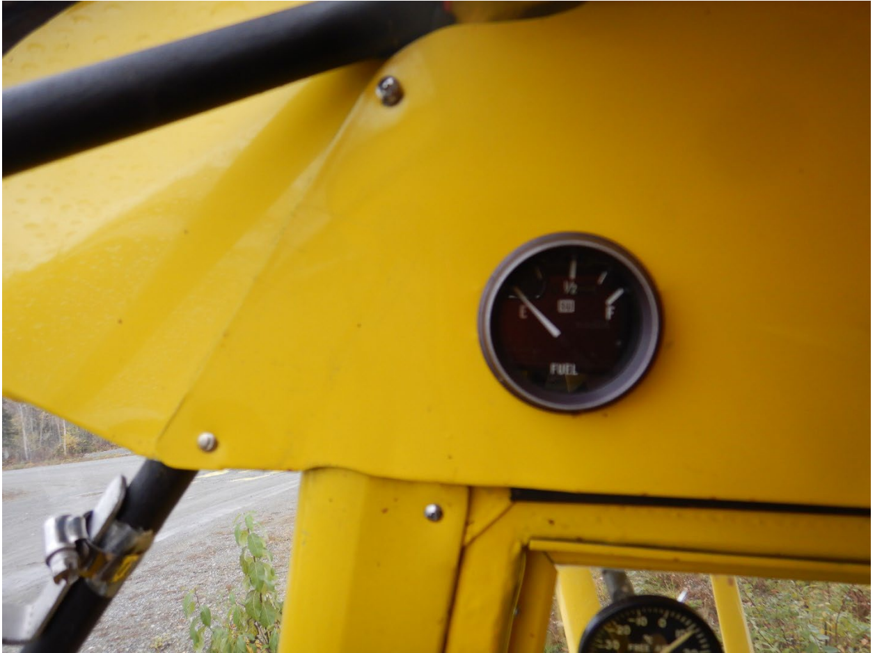
Figure 2. Right wing fuel tank gauge.
