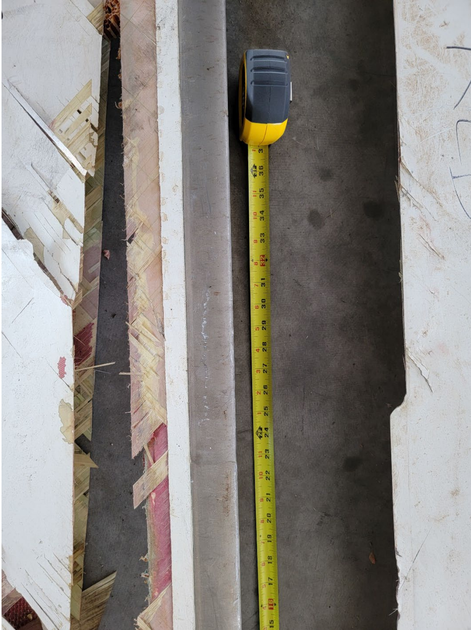
Figure 15 Witness marks on green rotor blade with white paint transfer from impact with heli utility basket.
