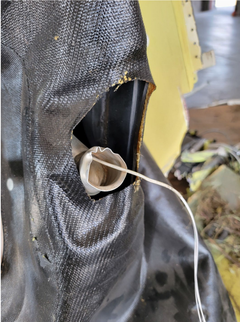
Figure 22 Bottom of main fuel cell. Forward fuel tank connection.
