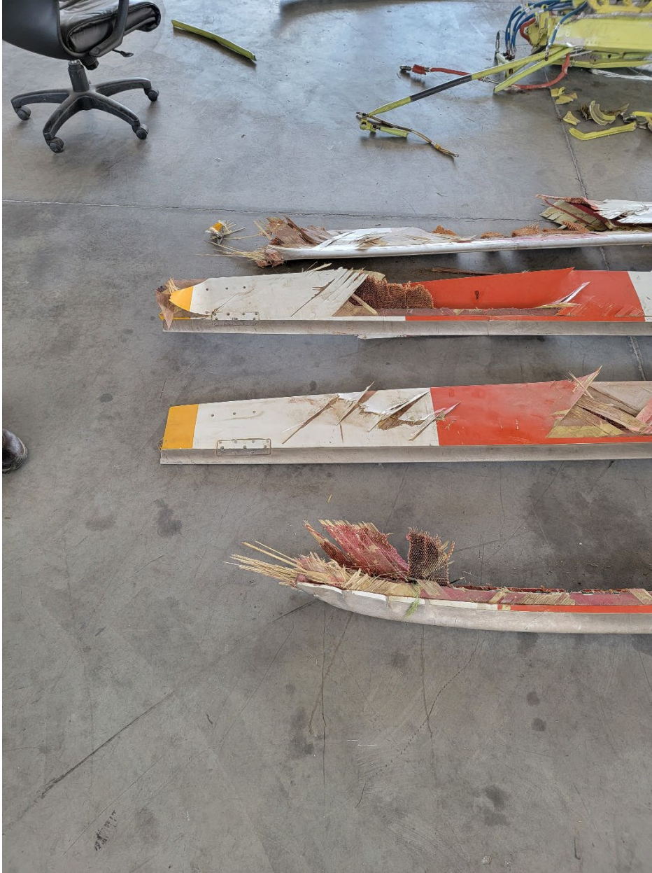
Figure 25 Top side tip damage to main rotor blades.
