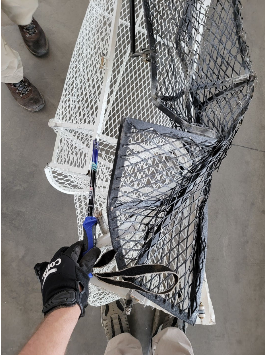
Figure 18 View of heli utility basket with broken ski pole.
