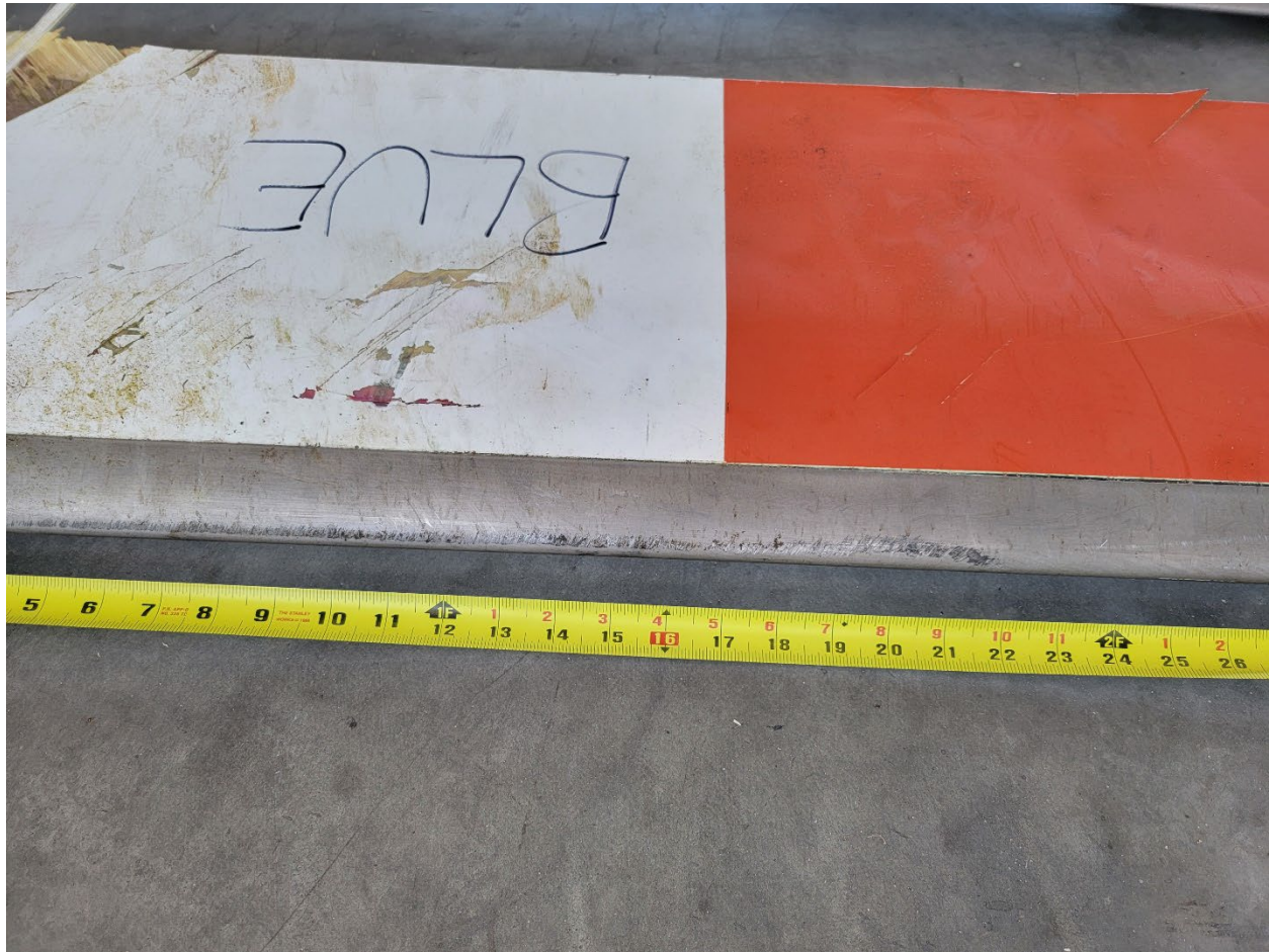
Figure 16 Witness marks on blue rotor blade with black paint transfer from impact with heli utility basket.
