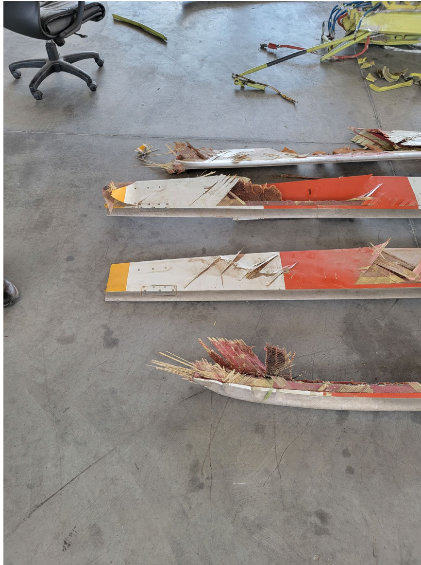
Photograph 3 - Main rotor blade tip damage (Courtesy of NTSB)
