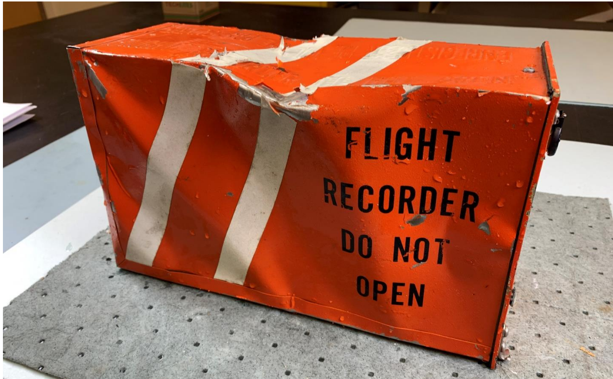
Figure 1. The L3 A-100S CVR, as received.
